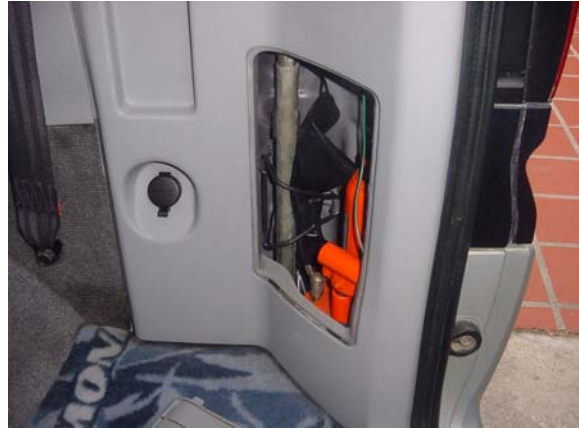
Figure 7: Jack and tools for changing tyre. Extra socket for 12 V power also visible (round black cap) - takes cigarette lighter type fitting.
