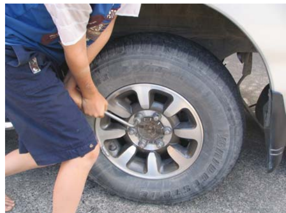
Figure 11: Undoing screws on wheel. Turn anti-clockwise to loosen, i.e. push down from this position.
