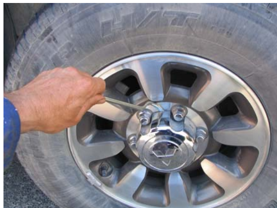
Figure 10: Remove plastic wheel cap, by prising with flat bar or screwdriver.
