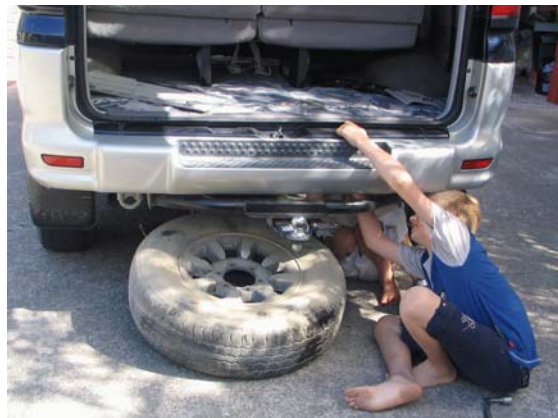
Figure 9: Releasing the spare wheel. Slide it out backwards.
