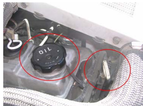
Figure 26: Oil cap (left) and dip stick (right).
