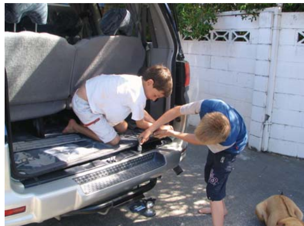
Figure 8: Lowering the spare wheel. Use the socket spanner to turn the bolt head anti-clockwise.
