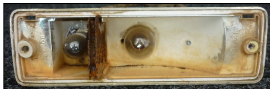
There is almost no silver reflector remaining and the divider panel is rusted quite badly, so were the globe and sockets
