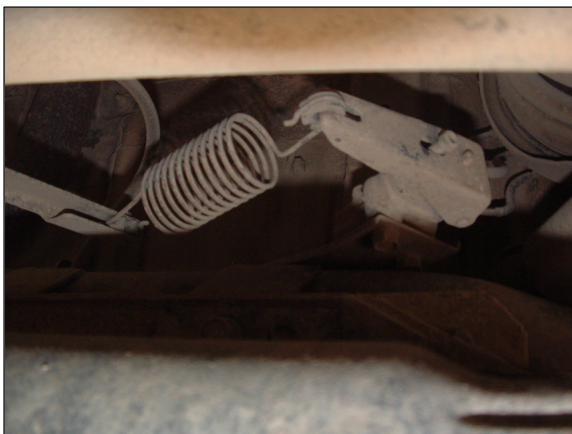
The two pictures above are from a stock standard GU4, you can see clearly how the spring is almost at a 45 degree angle to the BPV lever.
