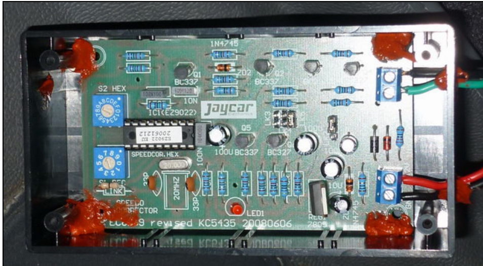
Mine mounted in the box just before the lid goes on The red silicon is to stop it from vibrating too much
