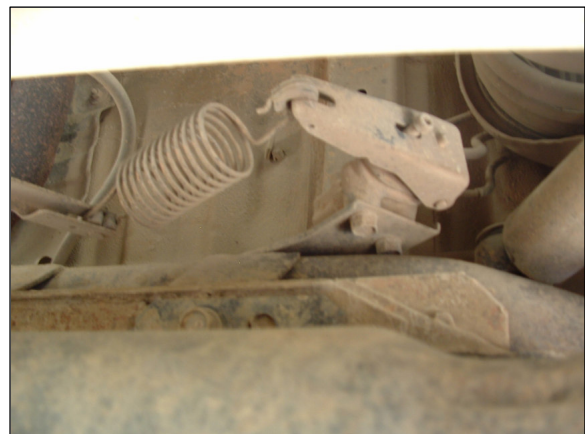
The two pictures above are from a stock standard GU4, you can see clearly how the spring is almost at a 45 degree angle to the BPV lever.
