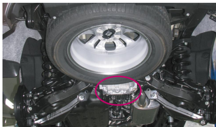
Use the DIFFERENTIAL as the Jacking Point
