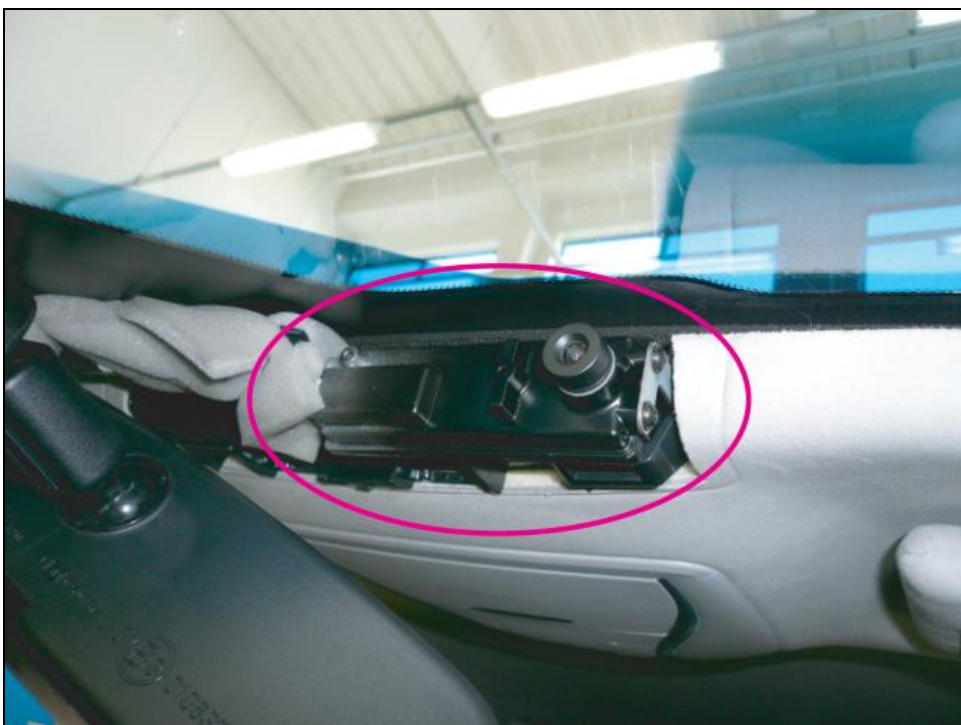
Lane Camera Unit (covers removed)
