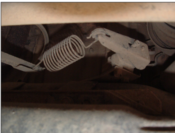
The two pictures above are from a stock standard GU4, you can see clearly how the spring is almost at a 45 degree angle to the BPV lever.
