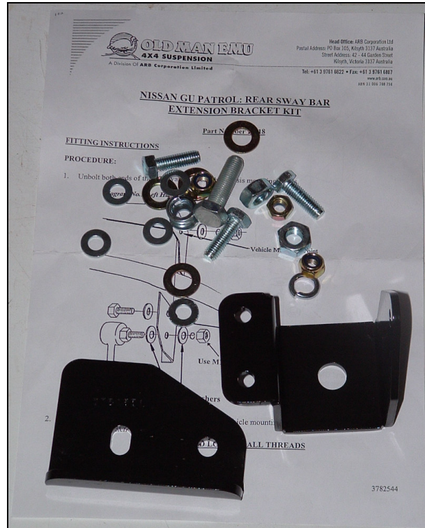
GU Rear Sway-Bar Extension Bracket Kit P/N: FK18
