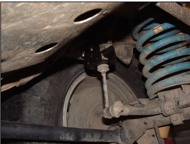
Right hand bracket installed
