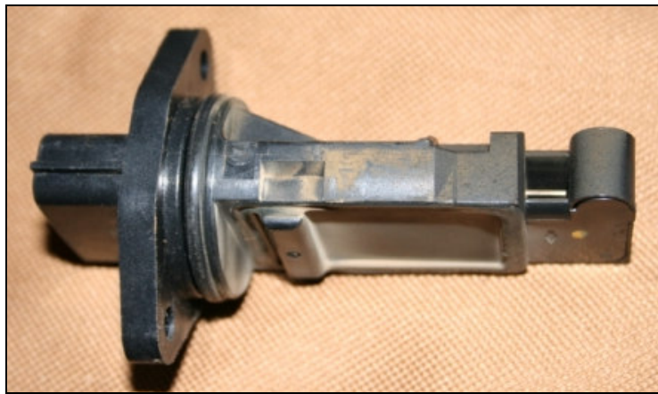
Early MAF, these have a circular entry point into the air duct. GU4 MAFs have a rectangular entry point and can only be inserted one way.
