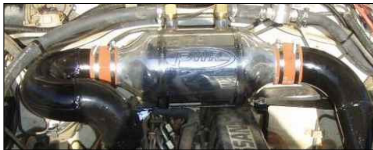
Aftermarket PWR air to liquid intercooler
