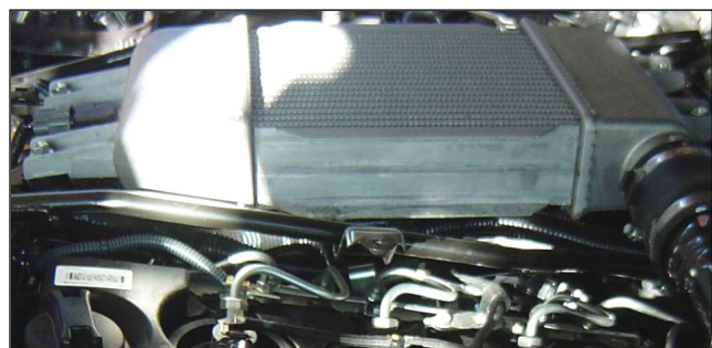
ZD30 CRD top mount air to liquid intercooler
