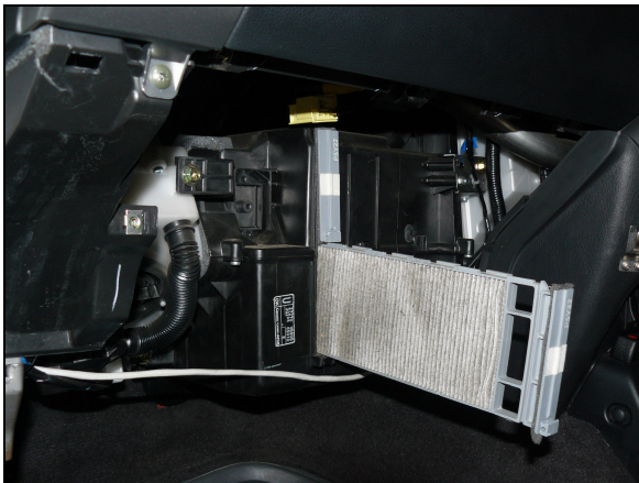
A dirty filter ready for a clean after 10,000klms
