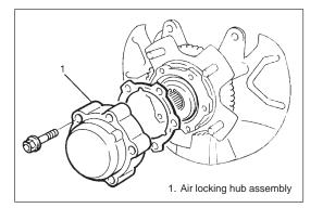
5) Remove air locking hub assembly (for 4WD).
