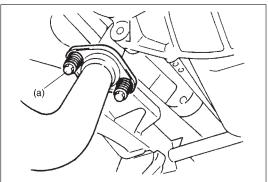
2) Tighten right and left engine mounting bracket bolts to specified torque.
