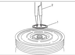
4) Install snap ring (1) using special tool.
