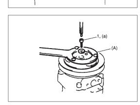
6) Tighten new clutch plate bolt (1) as specified torque.
