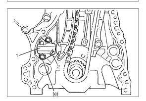
9) Install timing chain tensioner adjuster assembly (1) with a retainer (2).
