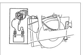
2) Connect battery to condenser cooling fan motor as shown in figure, then check that the condenser cooling fan motor operates smoothly.
