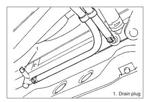
3) Drain coolant by loosening drain plug (1).
