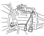
1. A/T output shaft speed sensor – input/turbine speed sensor coupler
