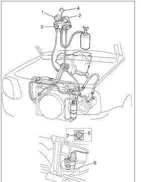
8) After the system has been charged with specified amount (500 - 600 g) of refrigerant or when low pressure gauge (1) and high pressure gauge (2) have indicated the following specified amount, close low pressure side valve (3) on manifold gauge set (4). At this time, look into the sight glass (5) of receiver/dryer (6) and check that there are no bubbles (7) in it, which means that the system is fully charged.
