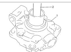
5) Remove lip type seal from front head (1) using bearing remover (2).
