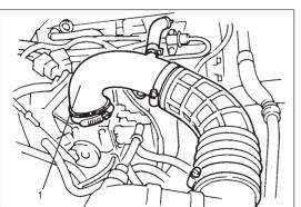
4) Disconnect air cleaner outlet NO.2 hose (1) from throttle body.
