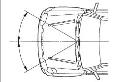
The air bag system is designed to activate only in severe frontal collisions. It is not designed to activate in rear impacts, side impacts, rollovers, or minor frontal collisions, since it would offer no protection in those types of accidents.
