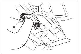
2) Install seal ring and install exhaust pipe (1) to exhaust manifold. Before installing seal ring, check it for deterioration or damage, and replace as necessary. Tighten pipe fasteners to specified torque.
