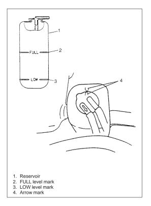
6) Add coolant to reservoir so that its level aligns with Full mark. Then, reinstall cap aligning arrow marks on reservoir and cap.
