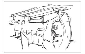
7) Remove bolts and nuts fastening engine cylinder block and transmission case and separate transmission from engine.8) Take down transmission.
