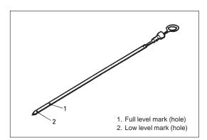
8) Start engine and run it for three minutes. Stop it and wait five minutes before checking oil level. Add oil, as necessary, to bring oil level to FULL level mark on dipstick.
