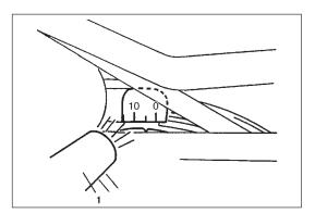
6) Using timing light (1), check that ignition timing is within specification.
