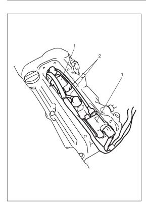
5) Install high-tension cords (2) to spark plugs and ignition coil assemblies (1) while gripping each cap.
