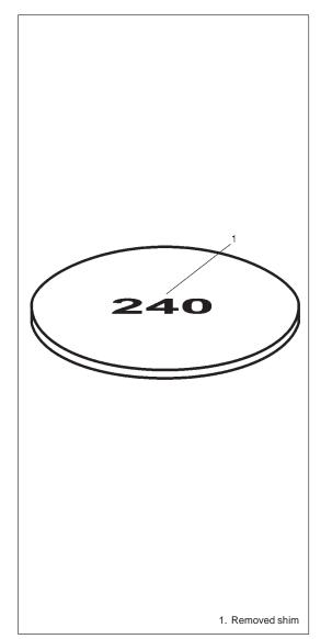
5) Check removed shim for No. (1) and determine replacement shim by calculating shim No. with the following formula and table.
