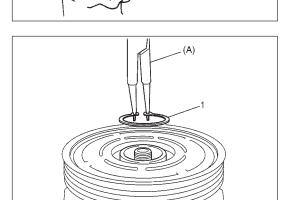
4) Remove circlip (1) using special tool.
