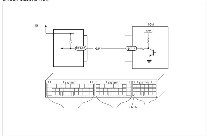
The serial data line is pulled up to about 12 V by ECM and TCM transmits information to ECM through it by controlling its grounding.
