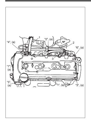
3) Install cylinder head cover to cylinder head.
