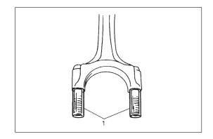
Install guide hoses (1) over connecting rod bolts. These guide hoses protect crank pin and threads of rod bolt from damage during installation of connecting rod and piston assembly.
