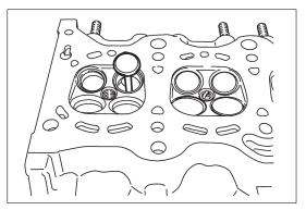
Install valve to valve guide.
