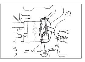
3) Loosen oil filter by using oil filter wrench (special tool).
