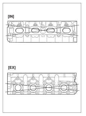
• Distortion of manifold seating faces: Check seating faces of cylinder head for manifolds, using a straightedge and thickness gauge, in order to determine whether these faces should be corrected or cylinder head replaced.
