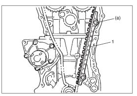
5) Apply engine oil to sliding surface of timing chain No.1 guide (1) and install it as shown in figure.
