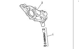
4) Install relief valve component (1) to rotor plate (2).
