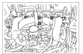
13) Remove intake manifold (1) with throttle body (2) and EGR pipe (3) from cylinder head (4), and then its gasket.
