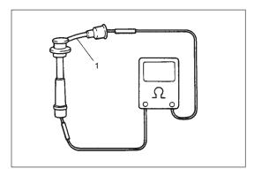
3) Measure resistance of high-tension cord (1) by using ohmmeter.
