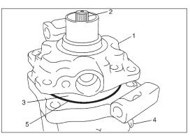
3) Remove front head (1) by pushing compressor shaft (2).
