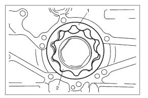
2) Remove outer rotor (1) and inner rotor (2).
