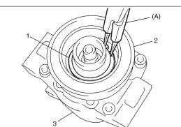
7) Remove snap ring (1) using special tool.
