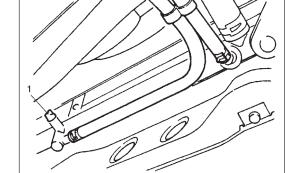
5) Fill radiator with specified amount of coolant, and run engine for 2 or 3 minutes at idle. This drives out any air which may still be trapped within cooling system. STOP ENGINE. Add coolant as necessary until coolant level reaches the filler throat of radiator. Reinstall radiator cap.
