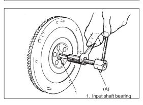
4) Use bearing remover (special tool) for pulling out of input shaft bearing.
