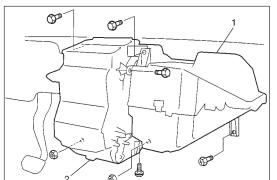
7) Remove cooling unit (1) with heater unit (2) from vehicle body.8) Remove cooling unit (1) from heater unit (2).
