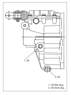
4) Torque drain plug and level/filler plug as specified below after applying sealant to its thread.
