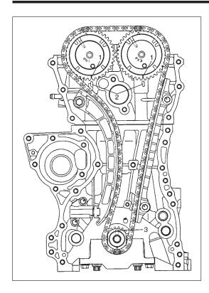
10) Apply engine oil to timing chain and then turn crankshaft clockwise by 2 revolutions and check that match marks (1) on intake and exhaust camshaft timing sprockets are in match with notches (2) on cylinder head and key(3) is on upside of crankshaft as shown in figure.
