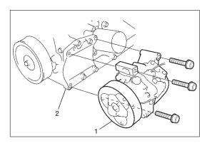
7) Remove compressor (1) from its bracket (2).
