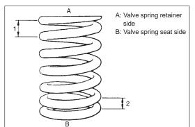
7) Install valve spring and spring retainer. Each valve spring has top end (large-pitch end (1)) and bottom end (small-pitch end (2)). Be sure to position spring in place with its bottom end (small-pitch end) facing the bottom (valve spring seat side).
