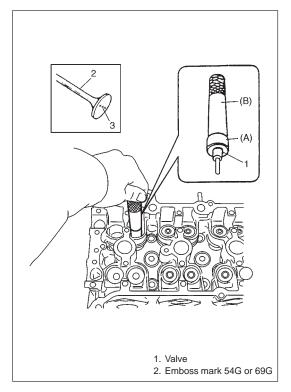
5) Install new valve stem seal (1) to valve guide.
