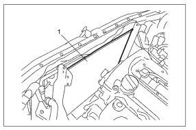
27) Install board (1) or the like on A/C condenser. This prevents damage to condenser fins when lifting and lowering engine assembly.
