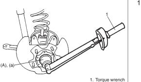
10) Tighten wheel bearing lock nut to specified torque while turning wheel hub by hand.
