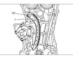
6) Apply engine oil to sliding surface of chain tensioner (1) and install chain tensioner and spacer.
