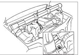
6) Lower engine and tighten engine mounting bracket bolts to specified torque.
