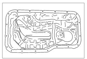
• Clean sealing surface on oil pan and cylinder block. Remove oil, old sealant and dust from sealing surface.
