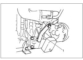
12) Remove intake manifold stiffener (1).
