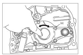
5) Install rotor plate and tighten all bolts to specified torque. After installing plate, check to be sure that rotors turn smoothly by hand (0.3 N·m (0.03 kg-m, 0.25 lb-ft) torque or below).
