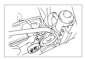
12) With hose connected, detach P/S pump from its bracket (if equipped) referring to Section 3B1.
