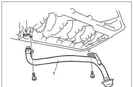
6) Remove oil pan and then oil pump strainer (1) from cylinder block.
