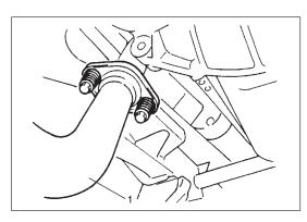
5) Disconnect exhaust pipe (1) from exhaust manifold.
