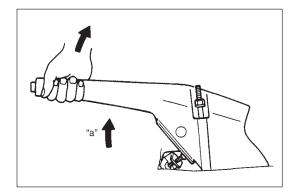
2) Check parking brake lever for proper operation and stroke, and adjust it if necessary.
