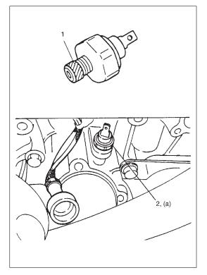
6) Before reinstalling oil pressure switch (2), be sure to wrap its screw threads with sealing tape (1) and tighten switch to specified torque.
