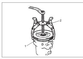
6) Remove magnet clutch pulley (1) by using a puller (2).
