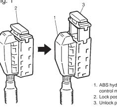
1. ABS hydraulic unit/ control module connector 2. Lock position
