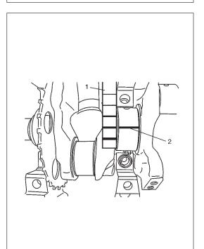
5) Remove bearing caps and using scale (1) on gaging plastic (2) envelop, measure gaging plastic width at its widest point. If clearance exceeds its limit, replace bearing. Always replace both upper and lower inserts as a unit.
