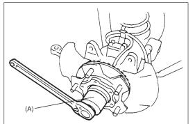
Uncaulk front wheel bearing lock nut (for 4WD).
