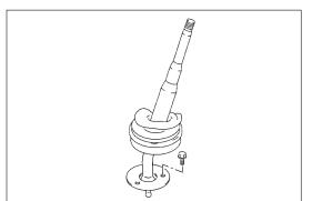
3) Remove 3 bolts, and then remove shift lever case plate and shift lever.
