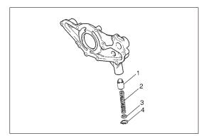
3) Remove relief valve (1), spring (2) and retainer (3) by removing circlip (4).
