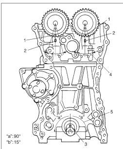
4. Camshaft (IN and EX) allowable turning range..... By marks on camshaft timing sprocket within 15° from notches on cylinder head on both right and left.
