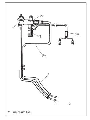
1) Install injector (3) and fuel pressure regulator (4) to special tool (injector checking tool).
