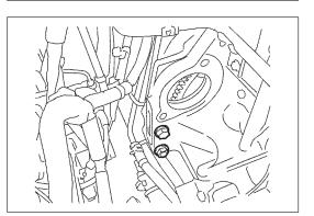
26) Remove bolts and nuts fastening cylinder block and transmission.
