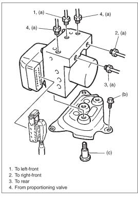
5) Remove three bolts and take out ABS hydraulic unit/control module assembly from bracket.
