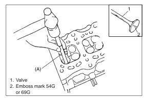
6) Using special tool (valve guide remover), drive valve guide out from combustion chamber side to valve spring side.
