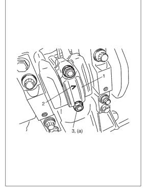
4) Install piston and connecting rod assembly into cylinder bore. Use special tool (Piston ring compressor) to compress rings. Guide connecting rod into place on crankshaft.
