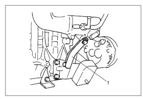
12) Remove intake manifold stiffener (1).
