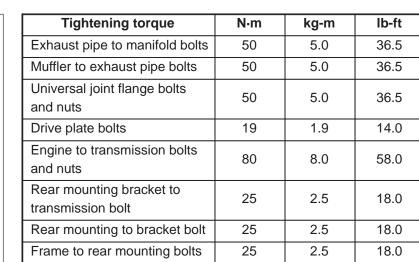
For remounting, reverse dismounting procedure. Use specified torque as given below and left.
