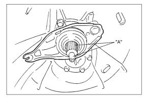
Slightly apply grease to input shaft. Then join transmission with engine. Refer to TRANSMISSION REMOUNTING of Section 7A.
