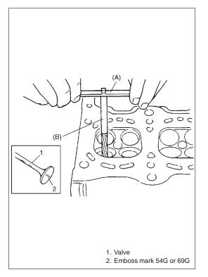
3) Ream valve guide bore with special tool (6.0 mm reamer for engine equipped with 69G type valve or 5.5 mm reamer for engine equipped with 54G type valve). After reaming, clean bore.
