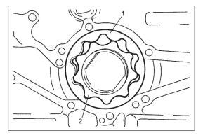
• Check relief valve (1) for excessive wear or damage and operates smoothly.
