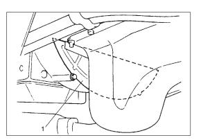
23) Remove clutch housing (torque converter housing for A/T) lower plate (1).
