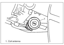
4)Remove coil antenna.
