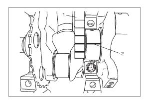
5) Using scale (1) on gaging plastic (2), check bearing clearance with newly selected standard bearing.
