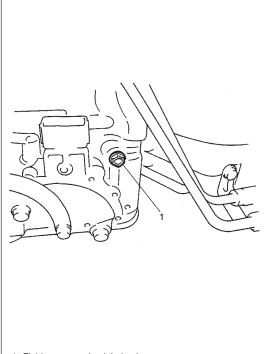
4) Depress foot brake fully, run engine at idle and stall then check fluid pressure in "D" or "R" range.
