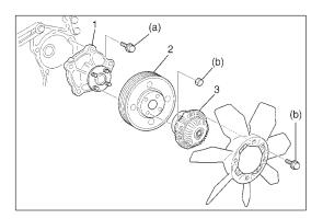
2) Install water pump (1) to cylinder block.
