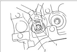
5) Remove valve stem seal (1) from valve guide and then valve spring seat (2).
