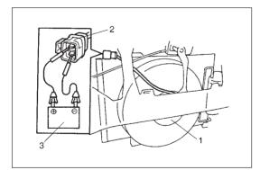
Connect battery (3) to A/C condenser fan motor coupler (2) as shown in figure, then check that the A/C condenser fan motor (1) operates smoothly.
