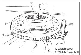
3) Install flywheel to crankshaft and tighten bolts applied with sealant at thread part to specification.
