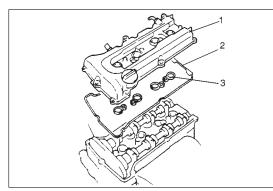
Remove cylinder head cover (1) with cylinder head cover gasket (2) and spark plug hole gasket (3).
