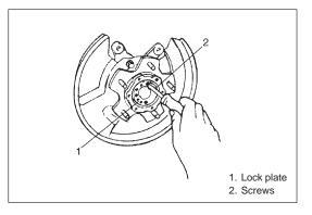
6') Remove front wheel bearing lock plate by loosening 4 screws (for 2WD).
