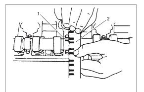
Remove housing, and using scale (2) on gaging plastic (1) envelop, measure gaging plastic width at its widest point.
