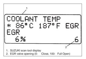
5) With engine idling (without depressing accelerator pedal), open EGR valve by using "STEP EGR" mode in "MISC TEST" menu. In this state, according as EGR valve opening increases engine idle speed drops. If not, possible cause is clogged EGR gas passage, stuck or faulty EGR valve, poor performance of ECT sensor or TP sensor or DTC and/or pending DTC is (are) stored in ECM memory.
