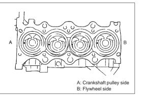
3) When installing piston and connecting rod assembly into cylinder bore, point front mark on piston head to crankshaft pulley side.
