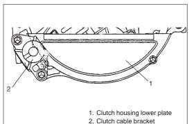
6) Remove clutch cable bracket and remove clutch housing lower plate from transmission case.
