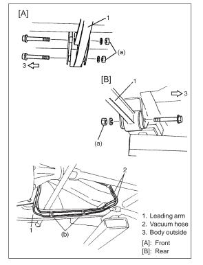
6) Remove bushings by using hydraulic press and special tools.
