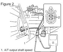
A/T output shaft speed sensor coupler
