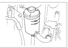
2) With engine stopped, check fluid level indicated on fluid tank or level gauge of tank cap, which should be between MAX and MIN marks. If it is lower than MIN, fill fluid up to MAX mark.
