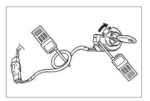
• Do not turn ON ignition switch with a radio antenna placed near coil antenna or its harness to Immobilizer Control Module. Or the system may detect abnormal condition and prevent engine from starting.
