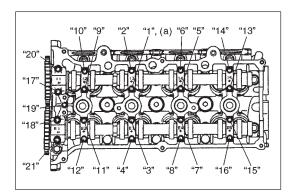
5) After applying engine oil to housing bolts, tighten them temporarily first. Then tighten them by the following numerical order in figure. Tighten a little at a time and evenly among bolts and repeat tightening sequence two or three times before they are tightened to specified torque.
