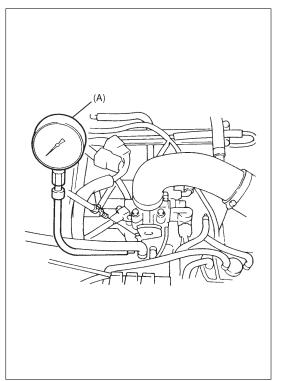
4) Connect special tool (Vacuum gauge) to intake manifold.
