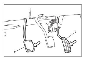
Disengage clutch (1) (to lighten starting load on engine) for M/T vehicle, and depress accelerator pedal (2) all the way to make throttle fully open.
