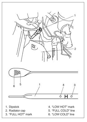
Pull out dipstick again and check fluid level indicated on it. Fluid level should be between FULL HOT and LOW HOT. If it is below LOW HOT, add an equivalent of DEXRON -IIE or DEX-RON -III, up to FULL HOT.
