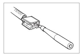
The adapter will also give an idea of whether contact tension is sufficient, helping to find an open or intermittent open due to poor terminal contact.
