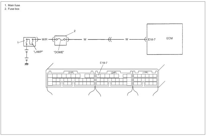
Battery voltage is supplied so that diagnostic trouble code memory, values for engine control learned by ECM, etc. are kept in ECM even when the ignition switch is turned OFF.
