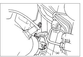
Install exhaust manifold stiffener (1).
