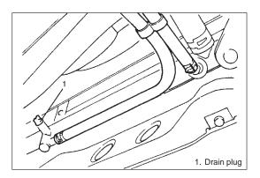
4) Drain coolant by loosening drain plug (1).
