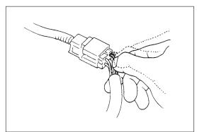
Poor terminal-to-wire connection. Check each wire harness in problem circuits for poor connection by shaking it by hand lightly. If any abnormal condition is found, change the wire harness assembly or component parts with new ones.
