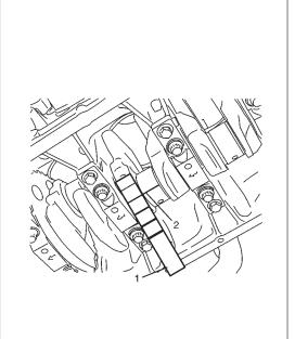
4) Install rod bearing cap (1) to connecting rod.
