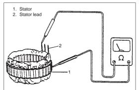
2) Using ohmmeter, check that there is no continuity between coil leads and stator core. If there is continuity, replace stator.
