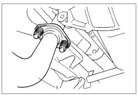
22) Disconnect exhaust pipe (1) from exhaust manifold.
