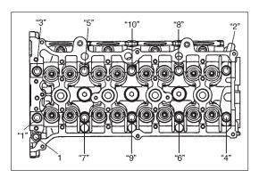
20) Loosen cylinder head bolts in such order as indicated in figure by using a 12 corner socket wrenches and remove them.
