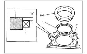
For oil seal installation, press-fit rear oil seal (1) to oil seal housing (2) by using special tool as shown in the figure.
