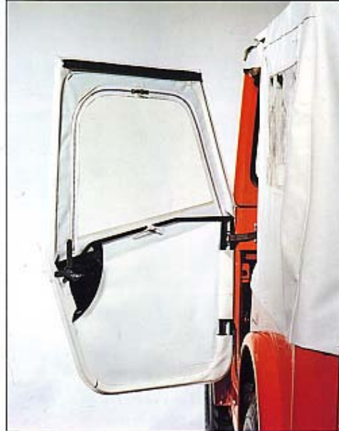
The Door, with Zipper Window for Easy Removing, is Designed for Quick Mounting or Dismounting.
