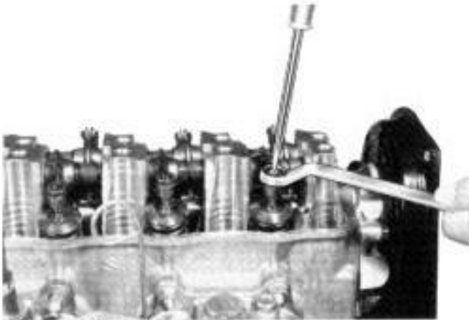
Fig. 3-152 Adjusting valve clearance
