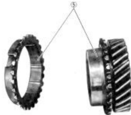
Fig. 13-21 ⑤ Checking contacting surface
