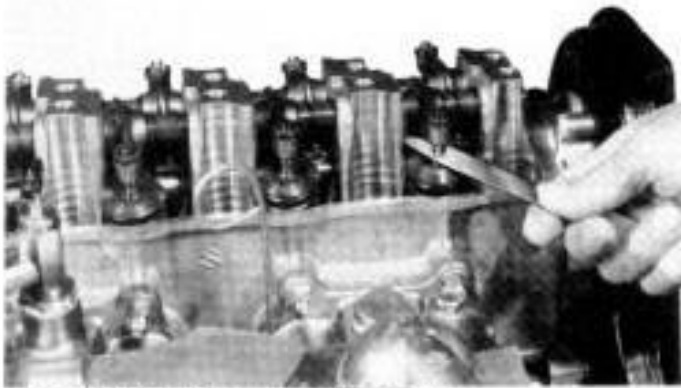
Fig. 3-151 Measuring valve clearance-
