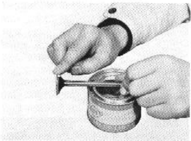
Fig. 3-69 Applying lapping compound to valve face
