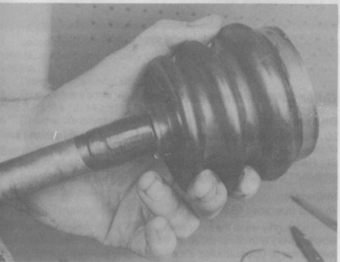
16.10 Wrap the splined area of the axle with tape to prevent damage to the boot when installing it
