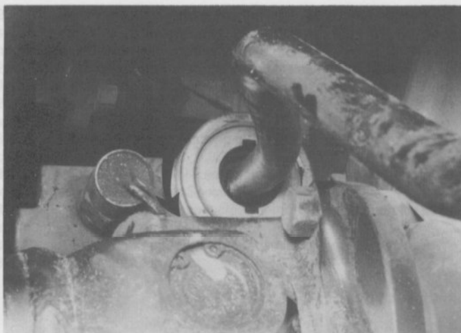
2.3 Push down on the lever guide while simultaneously twisting it counterclockwise
