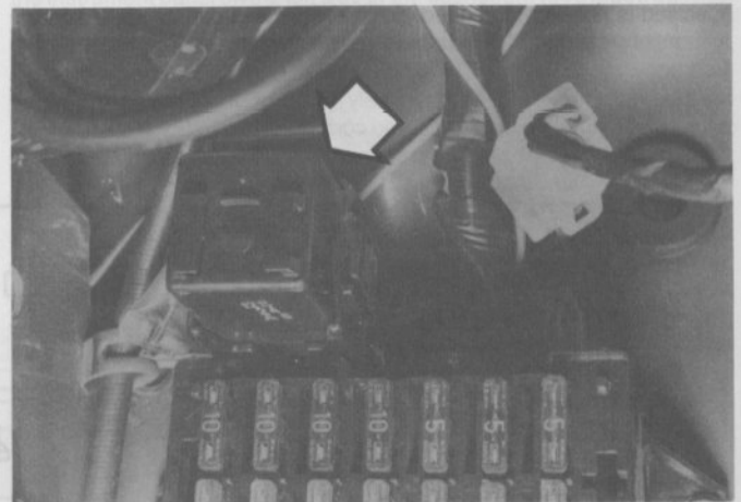
6.1 The turn signal and hazard flasher relay is located above the fuse box (Samurai)
