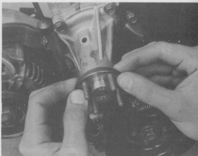
7.5 Try to rock the shaft up and down to check for play
