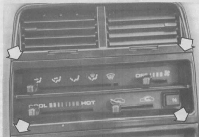
12.3c On Tracker and Sidekick models, gently grip the trim panel (arrows) and pull it off
