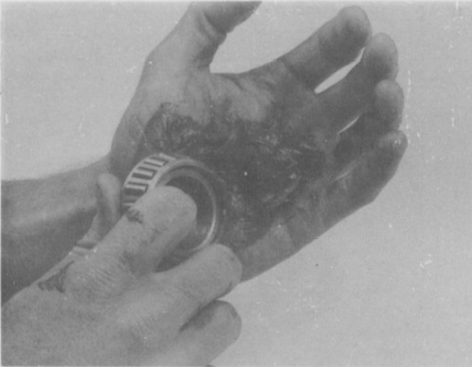
22.20 Work the grease into each bearing until it's full
