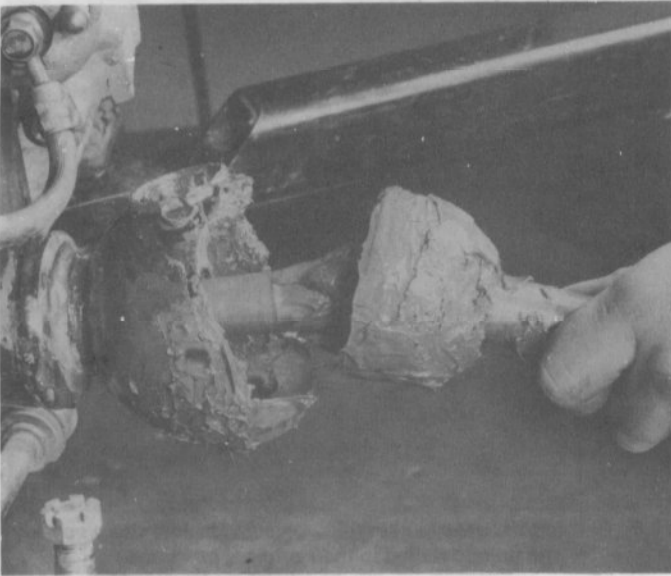
12.14 To remove the axleshaft, simply pull it out
