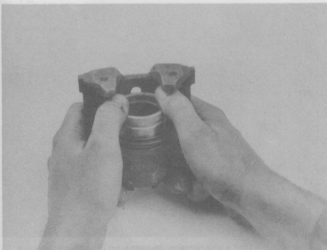
4.17 Position the piston squarely and push it straight into the caliper
