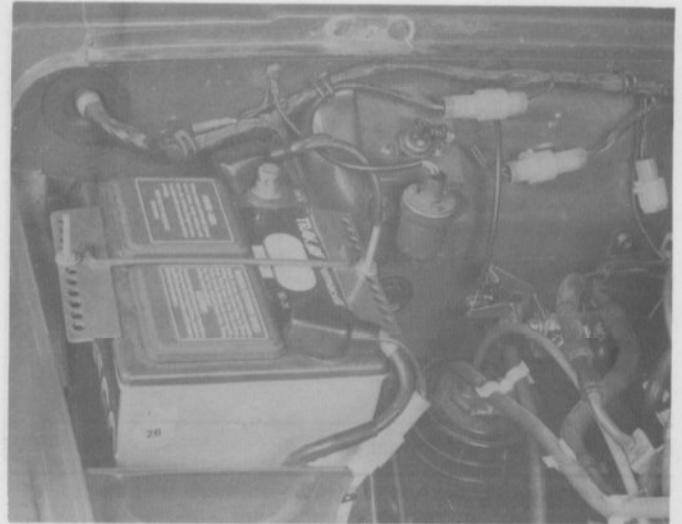
4.2 A fusible link protects the wire harness from overload and possible damage (Samurai)
