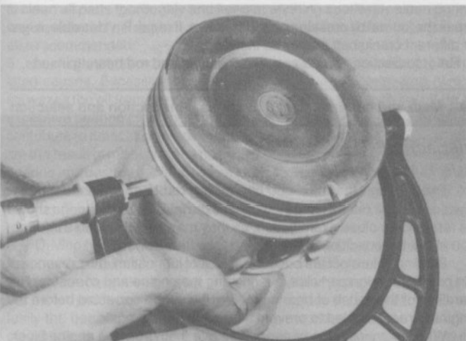
17.11b Measure the piston diameter at a 90-degree angle to the piston pin and make sure the micrometer is positioned the specified distance from the bottom edge of the skirt
