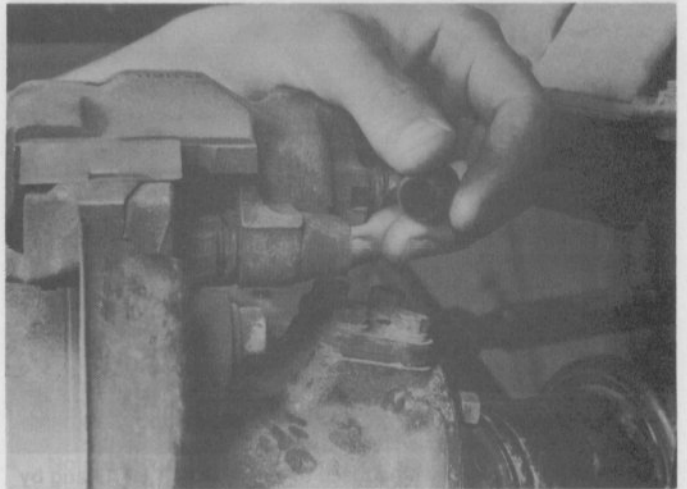
2.6c Remove the rubber caps to gain access to the caliper bolts
