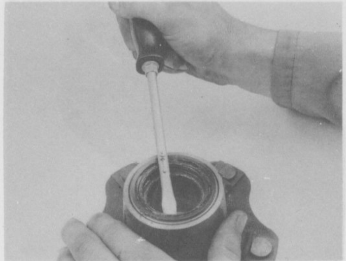
22.11 Use a screwdriver to pry the grease seal out of the hub
