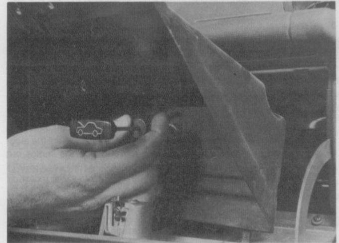
13.6 Remove the glove box with the hood latch cable
