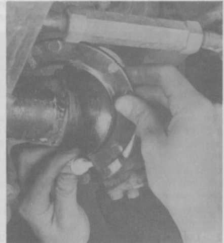
27.6 Apply some sealant to the ends of the seal retainers when installing them
