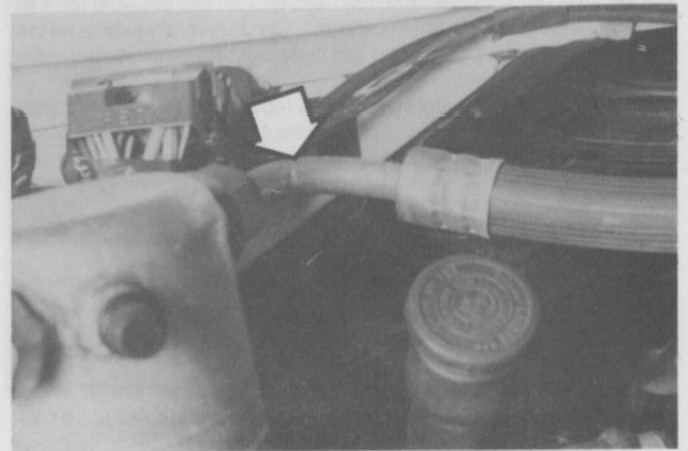
10.1 Air conditioning hoses are best identified by the metal tubes used at all bends (arrows) – DO NOT disconnect or accidentally damage the air conditioning hoses as the system is under high pressure
