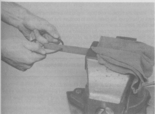
21.5 If the end gap is too small, clamp a file in a vise and file the ring ends (from the outside in only) to enlarge the gap slightly
