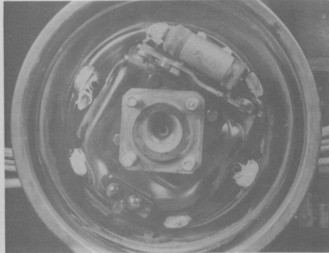
6.4m Lubricate the brake shoe contact areas with high-temperature grease
