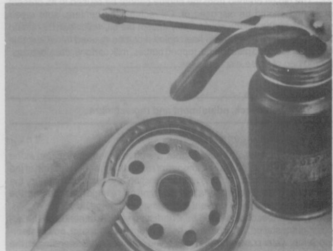
12.18 Lubricate the oil filter gasket with clean engine oil before installing the filter on the engine
