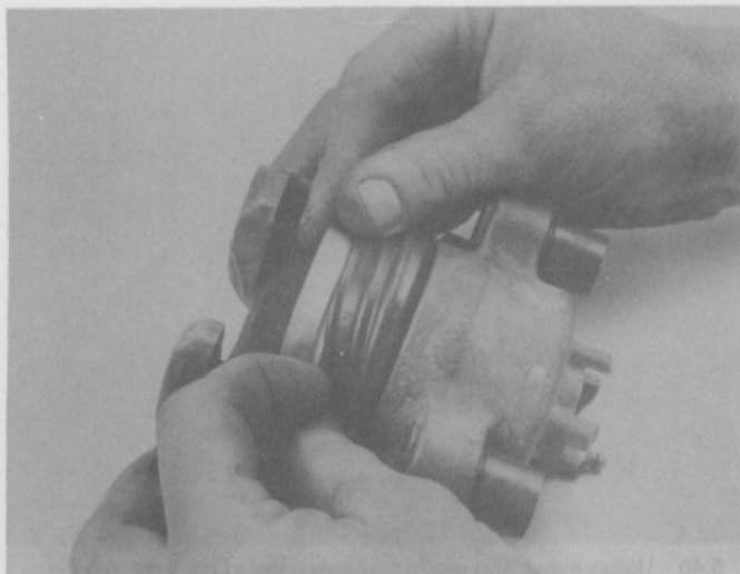
4.18 Install the lip of the dust boot in the groove on the piston
