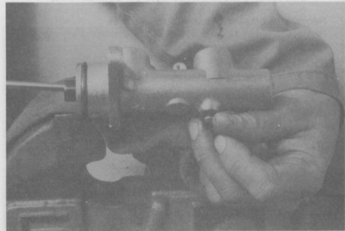
8.9 Push the pistons all the way in and remove the piston stop screw
