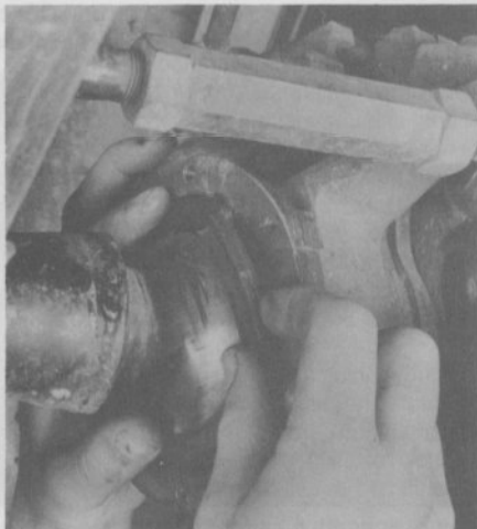
27.4 Cut the new seal, apply grease to the inside surface, and install it with the cut portion on top
