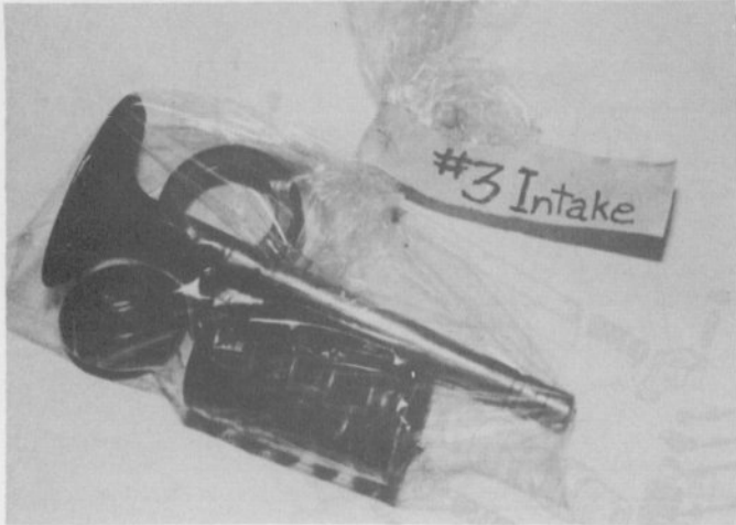
8.4 A small plastic bag, with an appropriate label, can be used to store the valve train components so they can be kept together and reinstalled in the correct guide
