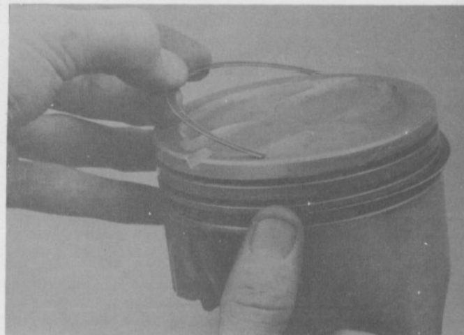
21.9b DO NOT use a piston ring installation tool when installing the oil ring side rails
