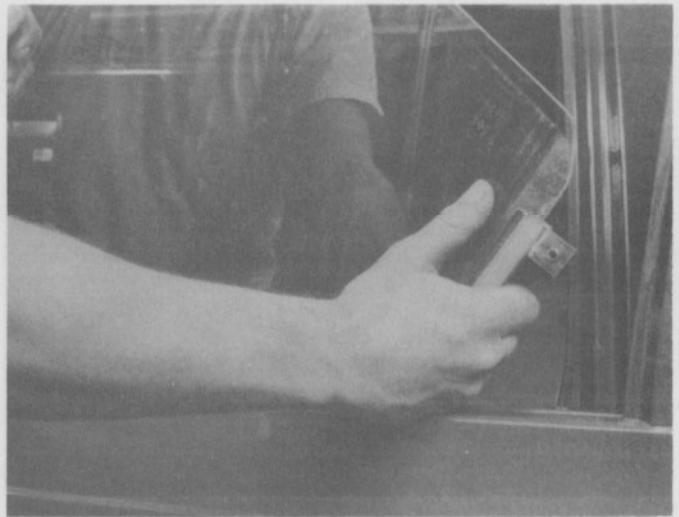
17.3b Remove the glass by carefully pulling it up – tilt it so it clears the channel
