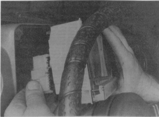
14.7 Press the locking tab on the electrical connector then unplug the connector from the instrument cluster
