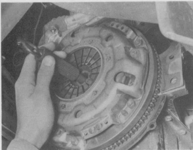
3.15 Center the clutch disc in the pressure plate with an alignment tool before the bolts are tightened – a clutch alignment tool can be purchased at most auto parts stores and eliminates all guesswork when centering the clutch disc in the pressure plate
