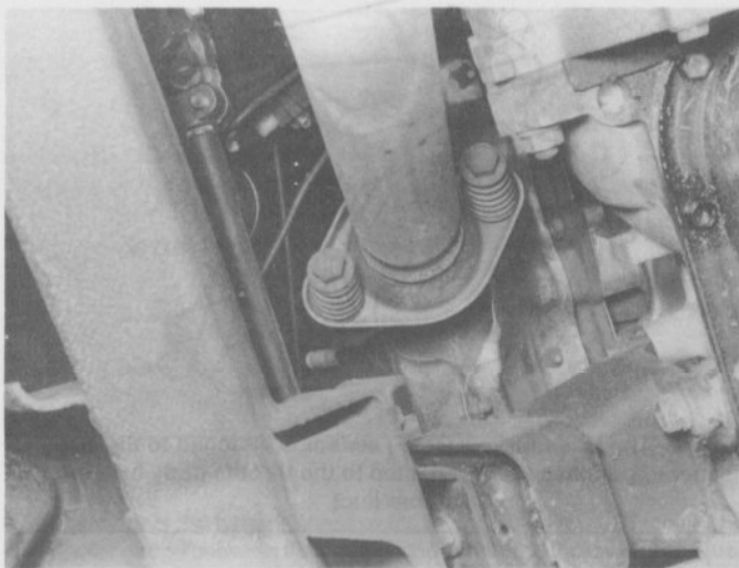
19.1b The exhaust pipe is connected to the exhaust manifold with two spring-loaded bolts—there is also a sealing ring or gasket (depending on the model) under the flange which should be replaced whenever the pipe is unbolted from the manifold
