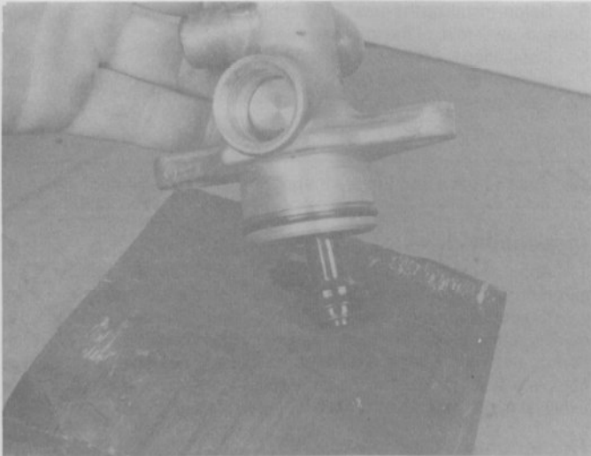
8.11b To remove the secondary piston assembly, tap the master cylinder firmly against a block of wood
