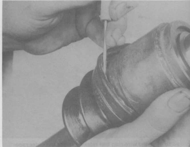
16.16 Equalize the pressure inside the boot by inserting a small, dull screwdriver between the boot and the outer race
