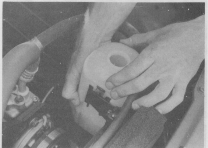
6.2 The coolant reservoir slips off/onto the bracket
