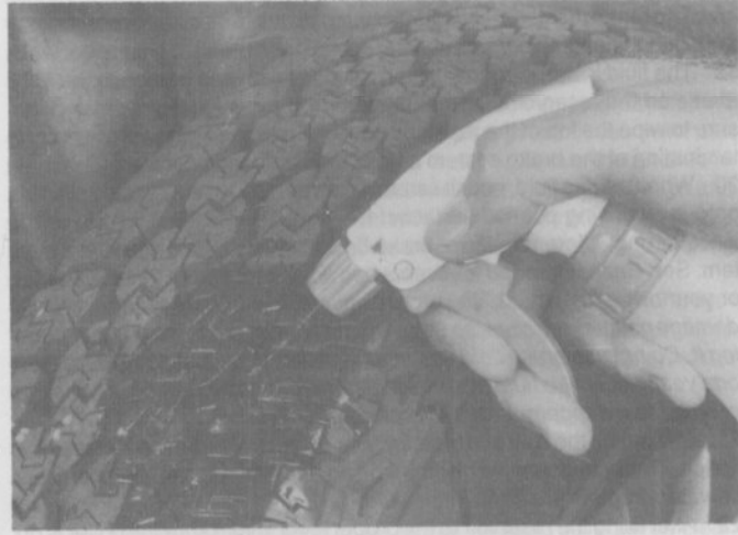
5.4b If the valve core is tight, jack up the low tire and spray a soapy water solution onto the tread as the tire is turned slowly – leaks will cause small bubbles to appear
