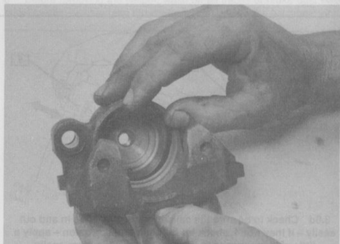
4.15 Push the new seal into the groove with your fingers, then check to see that it is not twisted or kinked
