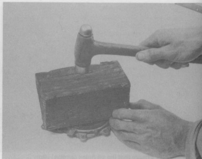
23.4 Drive the new seal into the housing with a block of wood or a section of pipe, if you have one large enough – make sure you don't cock the seal in the bore
