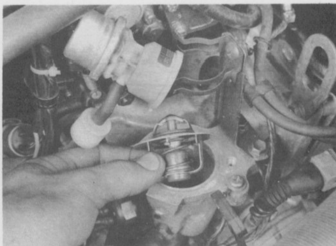
3.13 Install the thermostat, with the spring end down, into the stepped seat in the housing
