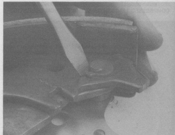
6.4j On Sidekick and Tracker models, pry the C-washer apart and remove it to separate the parking brake lever and adjusting lever from the rear shoe
