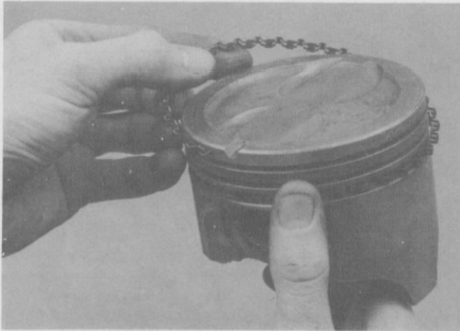
21.9a Installing the spacer/expander in the oil control ring groove
