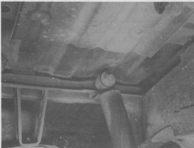
10.3a The upper end of the rear shock absorber on Samurai models mounts to a stud on the frame by a nut and washer
