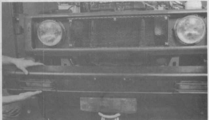
10.3 Support the bumper with a jack – place a wood block between the jack head and bumper
