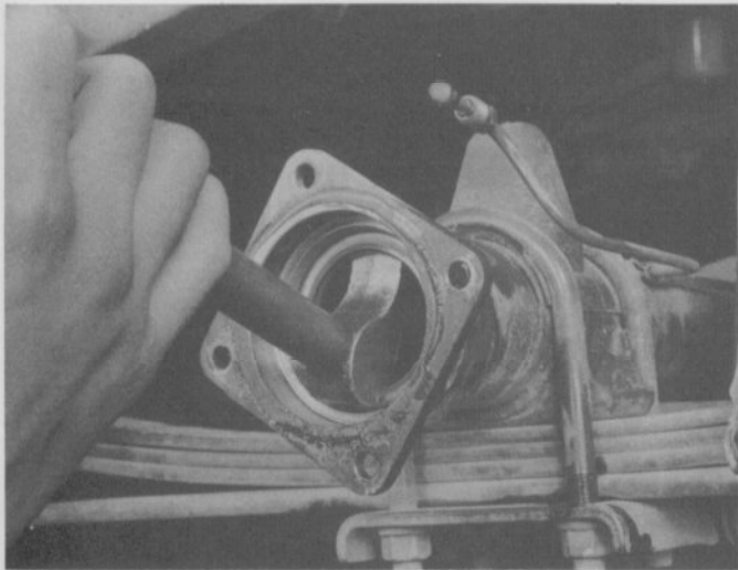
20.2 Pry out the seal, being careful not to damage the axle housing
