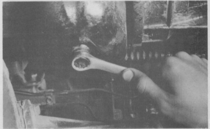
12.9 The oil drain plug is located at the bottom of the pan and should be removed with a socket or box-end wrench, as the corners on the bolt can be easily rounded off
