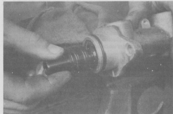
8.11a Remove the primary piston assembly from the master cylinder bore
