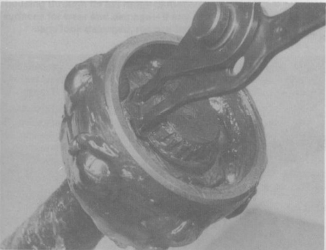
16.6 Remove the snap-ring from the end of the axle
