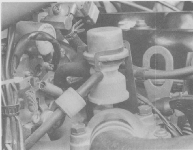
6.3a The MCV clips into a bracket near the thermostat housing
