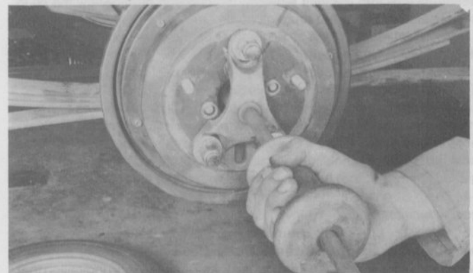
18.11 Use a slide hammer to remove stubborn brake drums
