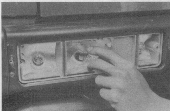
12.3 Push the bulb in and twist it counterclockwise to remove it – when installing the bulb, make sure the pins on the bulb line up with the proper slots in the socket
