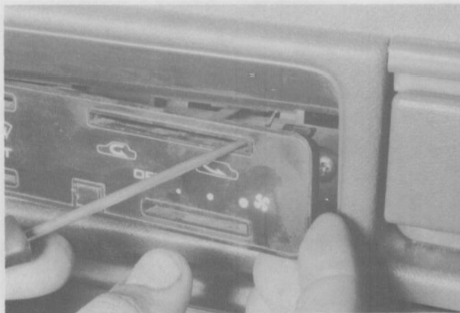
12.3a On Samurai models, slip an L-hook through the slotted openings and gently pull the faceplate off . . .
