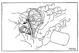
HINT: If the plunger does not spring out, press the slipper into the chain tensioner with a screwdriver or your finger so that the hook is released and the plunger springs out.
