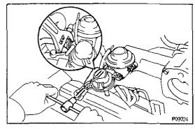
(b) Install the two nuts holding the EGR valve and air intake chamber.
