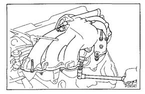
(d) Install two new gaskets and the air intake chamber with the four bolts and six nuts.
