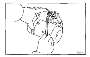
f) Connect the lead wire to terminal C, and install the nut.
