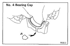
(b) Align the bearing claw with the claw groove of the main bearing cap, and push in the seven lower bearings.
