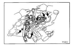
(c) Install the emission control valve set assembly with the four bolts.
