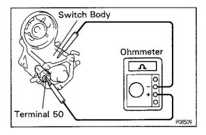
2. PERFORM HOLD—IN COIL OPEN CIRCUIT TEST
