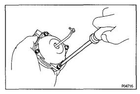
(c) If necessary, remove the four screws and disassembly the throttle valve diaphragm.
