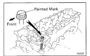
(c) Mark the front of the cylinder head bolt head with paint.
