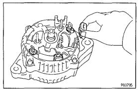
(b) Remove the four rubber insulators.
