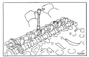
(h) Alternately and uniformly loosen and remove the No.4 and No.6 bearing cap bolts.
