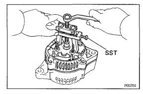
(b) Using SST, remove the rectifier end frame. SST 09286-46011
