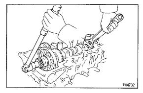
(c) Hold the intake camshaft with a wrench, remove the bolt and distributor gear.
