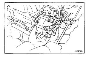
4. REMOVE DISTRIBUTOR CAP WITHOUT DISCONNECTING HIGH-TENSION CORDS
