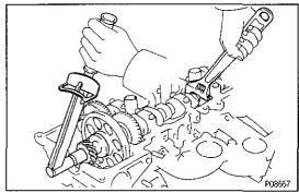
(c) Hold the intake camshaft with a wrench, install and torque the bolt.
