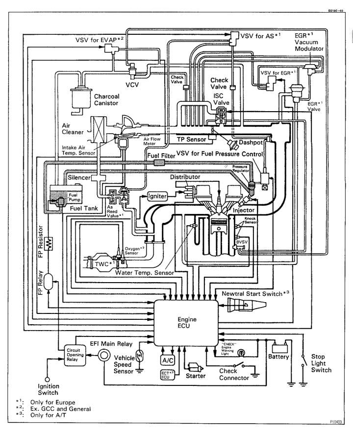
The EFI (Electronic Fuel Injection) system is composed of three basic sub-systems: Fuel, Air Induction and Electronic Control Systems.
