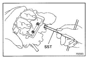
(b) Remove the primary and secondary main jets and gaskets.
