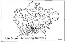
(c) Adjust turning the idle speed adjusting screw.
