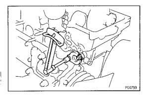
(c) Install the chain tensioner with the two nuts.
