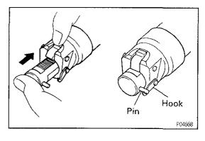
(b) Release the ratchet pawl, fully push in the plunger and apply the hook to the pin so that the plunger cannot spring out.
