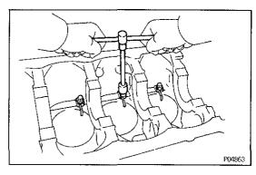
8. REMOVE CHECK VALVES AND OIL NOZZLES Remove the six check valves and oil nozzles.
