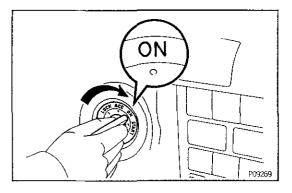
(b) Turn the ignition switch ON.
