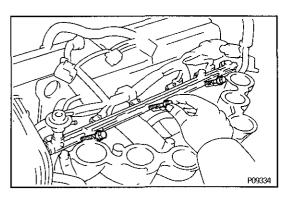
(g) Temporarily install the three bolts holding the delivery pipe to the intake manifold.
