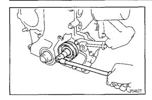
8. REMOVE DRIVE BELT IDLER PULLEY Remove the bolt and idler pulley.
