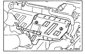
(b) Install the heat insulator with the three bolts.
