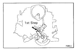
(2) Check that the fast idle lever is a set in the 1st step of the fast idle cam as shown.
