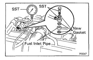
(d) Install the No.1 fuel pipe and SST (pressure gauge) to the delivery pipe with three new gaskets and SST (union bolt).
