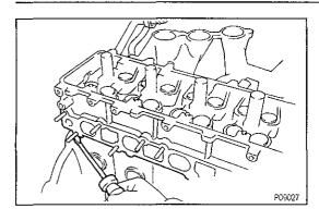
(c) Lift the cylinder head from the dowels on the cylinder block, and place the cylinder head on wooden blocks on a bench.
