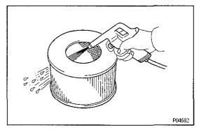
(e) Remove excess water by shaking the element or blowing with compressed air.
