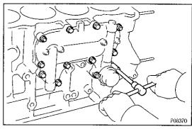
11. REMOVE OIL COOLER COVER AND OIL COOLER Remove the ten bolts, two nuts, oil cooler cover with the oil cooler and gasket.
