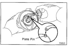
(b) Insert the vacuum advancer with the packing into the housing and position the advancer lever hole over the breaker plate pin.
