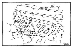
(b) Install the No.1 heat insulator and No.2 heat insulator with the six bolts.
