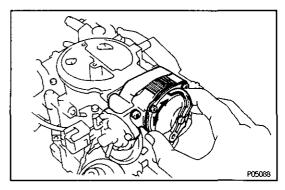
(b) Depending on vehicle operating conditions, turn the coil housing and adjust the engine starting mixture.
