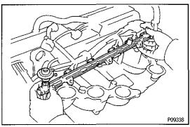
(f) Place the six injectors together with the delivery pipe in position on the intake manifold.
