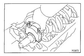
(b) Using the removed main bearing cap bolts, pry the main bearing cap back and forth, and remove the main bearing caps, lower bearings and lower thrust washers (No.4 main bearing cap only).
