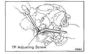
(c) Adjust by turning the TP adjusting screw.
