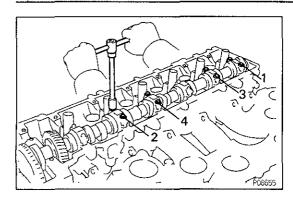
(d) Loosen and remove the No.3, No.4, No.6 and No.7 bearing cap bolts, alternately loosening the left and right bolts uniformly in several passes, in the sequence shown.
