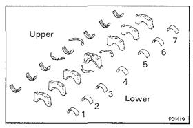
HINT: Arrange the main bearings and thrust washers in correct order.
