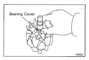
(b) Place the bearing cover on the rotor.
