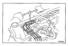
(g) Install the No.1 cord clamp mounting bolt.
