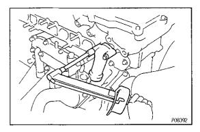
(e) Install the water by-pass outlet and pipe with the two bolts.
