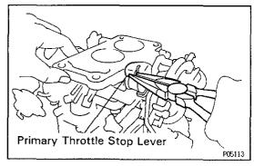
(b) Adjust by bending the primary throttle stop lever.
