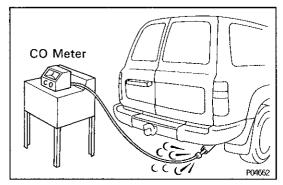
(c) Insert co Meter testing probe at least 40 cm (1.3 ft) into the tailpipe, during idling. Immediately check the co concentration at Idle.
