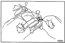
(b) Install the float and secure it with the pivot pin.
