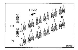
HINT: Arrange the valves, valve springs, spring seats and spring retainers in correct order.
