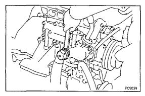
(b) Install the oil pressure switch.
