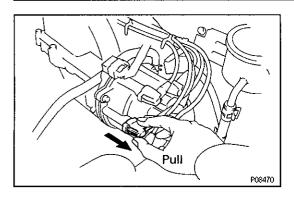
(c) Check that the lock claw of the holder is engaged by lightly pulling the holder.
