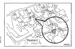
(b) Apply adhesive to the spark plug tube hole of the cylinder head.
