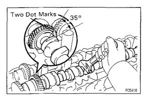
(c) Set the timing mark (two dot marks) of the camshaft driven gear at approx. 35° angle by turning the hexagon wrench head portion of the intake camshaft with a wrench.
