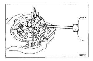
(c) Install the rectifier holder with the four screws.
