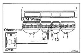
(c) Measure the resistance between each terminal of the wiring connectors.
