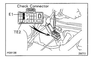
2. First using SST, connect terminals TE2 and E1 of the check connector.
