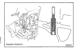
(g) Using a sharp 7 mm reamer, ream the guide bushing to obtain the standard specified clearance (See page EG-58) between the guide bushing and valve stem.
