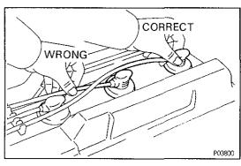
(b) Disconnect the high – tension cords at the rubber boot.
