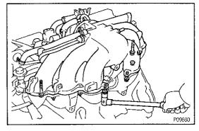
(c) Remove the four bolts, four nuts, air intake chamber and two gaskets.
