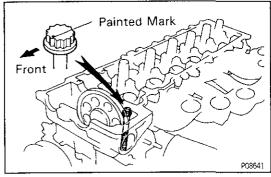
(c) Mark the front of the cylinder head bolt head with paint.
