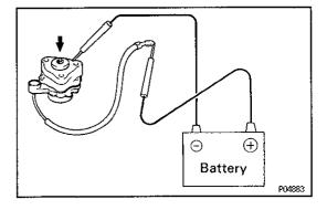
(d) Connect the OVCV body and wire terminal to the battery terminals and check that the valve is retracted.
