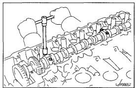
(f) Alternately and uniformly loosen and remove the No.2 and No.5 bearing cap bolts.
