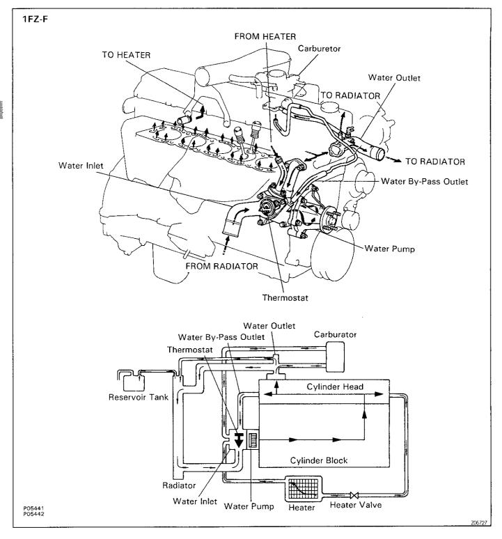
The cooling system is composed of the water jacket (inside the cylinder block and cylinder head), radiator, water pump, thermostat, cooling fan, hoses and other components.
