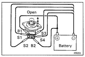
(b) Apply battery voltage to terminals B1 and B2, and while repeatedly grounding S4-S3-S2-S1-S4 in sequence, and check that the valve moves toward the open position.
