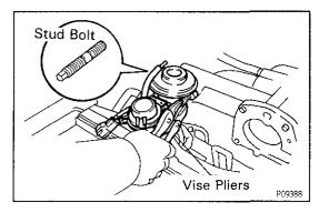
(d) Using vise pliers, remove the two stud bolts, EGR valve and vacuum modulator assembly and gasket.
