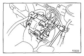
(c) Remove the hold-down bolt and distributor.
