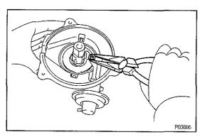
(c) Using needle-nose pliers, install the E-ring.
