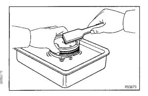
(c) Using solvent and a brush, thoroughly clean the piston.
