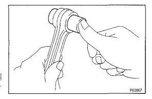
(e) Check the piston pin fit at normal room temperature. Coat the piston pin with engine oil, and push it into the connecting rod with your thumb.
