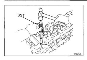
(b) Using SST and a hammer, tap out the guide bushing. SST 09201-15010
