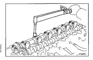
(I) Uniformly tighten the fourteen bearing cap bolts in several passes.
