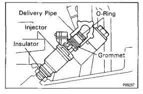
4. Install the injector to the delivery pipe and intake manifold as shown in the illustration.
