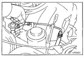
(c) When the fuel return hose is pinched, the pressure within high pressure line will rise to approx. 392 kPa (4 kgf/cm², 57 psi). In this state, check to see that there are no leaks from any part of the fuel system. NOTICE: Always pinch the hose. Avoid bending as it may cause the hose to crack.
