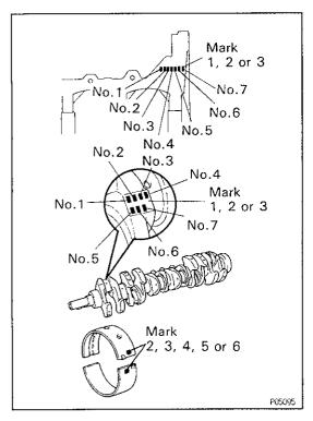
HINT: If using a standard bearing, replace with one having the same number. If the number of the bearing cannot be determined, select the correct bearing by adding together the numbers imprinted on the cylinder block and crankshaft, then selecting the bearing with the same number as the total. There are five sizes of standard bearings, marked "2", "3", "4", "5" and "6" accordingly.
