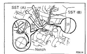
Using SST (A), press down the valve lifter and place SST (B) between the camshaft and valve lifter flange. Remove SST (A).
