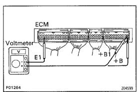
(b) Measure the voltage between each terminal of the wiring connectors.
