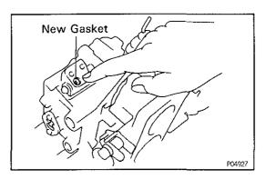
(c) Place a new gasket in position on the carburetor body.
