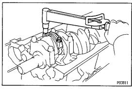
(h) Install the connecting rod cap with the two nuts. (See step 8 on page EG-164)
