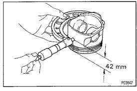
(a) Using a micrometer, measure the piston diameter at ring angles to the piston pin center line, 42 mm (1.65 in.) from the piston head.
