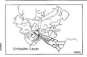
(b) Adjust by bending the unloader lever.
