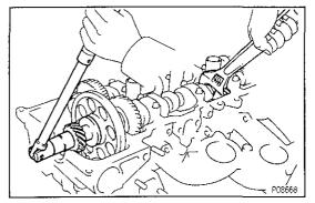
(c) Hold the intake camshaft with a wrench, remove the bolt and distributor gear.
