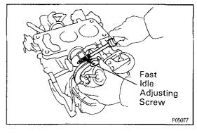
(d) Adjust by turning the fast idle adjusting screw.
