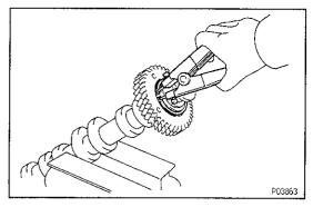
(c) Using snap ring pliers, install the snap ring.
