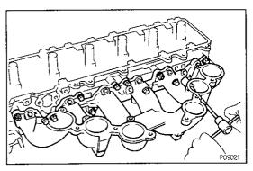
(b) Install the intake manifold with the six bolts and two nuts.
