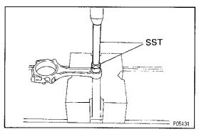
(c) Using SST and a press, press in the bushing. SST 09608-30012, (09608-04020), 09631-20031
