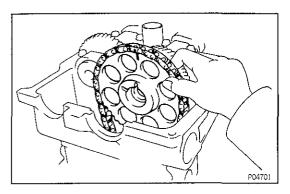
(d) Remove the camshaft timing gear and chain from the intake camshaft and leave on the slipper and damper.
