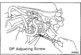
If the DP setting speed is not as specified, adjust the setting speed by turning the DP adjusting screw. Dash pot setting speed:
