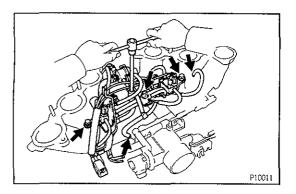
(c) Install the emission control valve set assembly with the four bolts.
