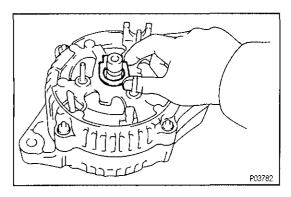
(c) Remove the seal plate.
