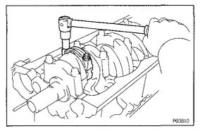
(b) Remove the connecting rod cap nuts.
