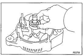
(c) Remove the thrust washer.
