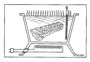
(e) Gradually heat the cylinder head to  $80 - 100^{\circ}$ C (176) — 212°F).
