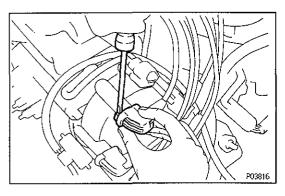
4. DISCONNECT HIGH—TENSION CORDS FROM DISTRIBUTOR CAP AND IGNITION COIL
