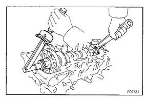
(c) Hold the intake camshaft with a wrench, install and torque the bolt.
