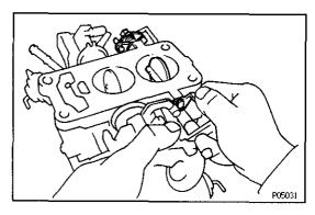
(c) Check the full opening angle of the secondary throttle valve.
