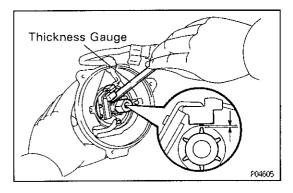
(c) Using a thickness gauge, adjust the gap between the signal generator projection with governor shaft projection.
