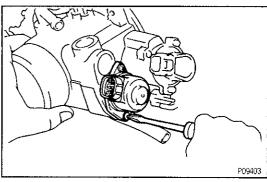
(b) Install the ISC valve with the two screws.
