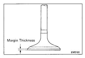
(c) Check the valve head margin thickness.
