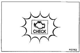
4. Read the diagnostic code as indicated by the number of flashes of the "CHECK" engine warning light.
