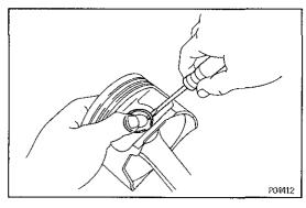
(e) Install a new snap ring on the other side of the piston pin hole.
