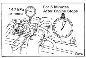
(q) Check that the fuel pressure remains as specified for 5 minutes after the engine is stops.
