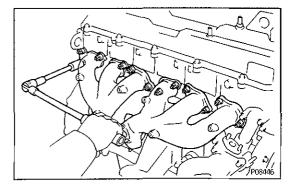
(b) Remove the 13 nuts, No.1 exhaust manifold, No.2 exhaust manifold and two gaskets.
