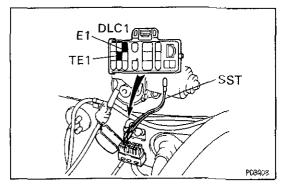
Using SST, connect terminals TE1 and E1 of the check connector
