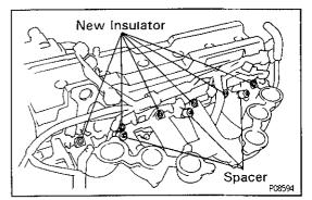
(e) Place six new insulators and the three spacers in position on the intake manifold.
