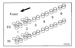
HINT: Arrange the valve lifters and shims in correct order.
