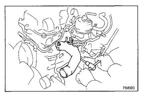
(c) Remove the two nuts, water outlet and gasket.
