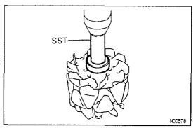
(c) Using SST and a press, press in a new bearing. SST 09820-00030
