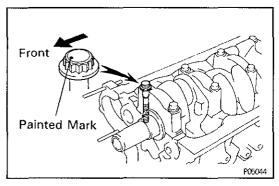
(c) Mark the front of the main bearing cap bolt with paint.
