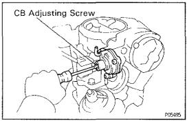
(d) Adjust by turning the CB adjusting screw.
