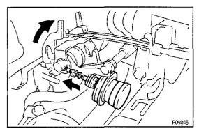
D. Check and adjust dashpot setting speed
