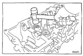
(d) Using a plastic—faced hammer, lightly tap the valve stem tip to assure proper fit.
