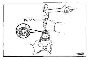
(c) Using a punch, stake the armature shaft.
