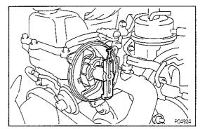
(b) Check that the distributor rotor direction is as shown.
