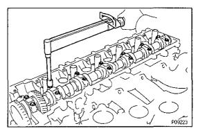
(j) Uniformly tighten the fourteen bearing cap bolts in several passes.
