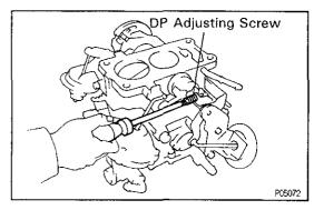
(c) Adjust by turning the DP adjusting screw.
