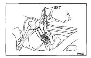
(j) Remove SST from the check connector. SST 09843-18020
