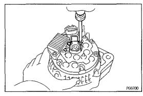
(b) Remove the two screws and brush holder.
