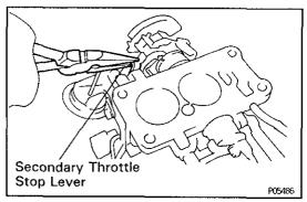
(d) Adjust by bending the secondary throttle stop lever.
