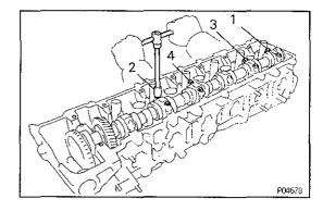
(d) Loosen and remove the No.3, No.4, No.6 and No.7 bearing cap bolts, alternately loosening the left and right bolts uniformly in several passes, in the sequence shown.
