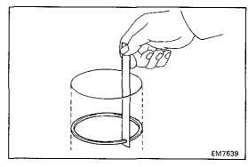
(c) Using a thickness gauge, measure the end gap.
