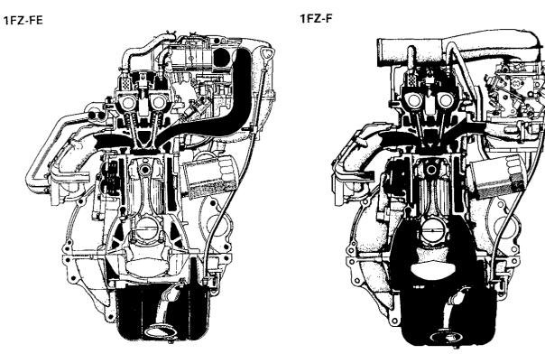
The 1FZ-FE and 1FZ-F engines are an in-line, 6-cylinder engine with the cylinders numbered 1-2-3-4-5-6 from front. The crankshaft is supported by 7 bearings inside the crankcase. These bearings are made of aluminum alloy.
