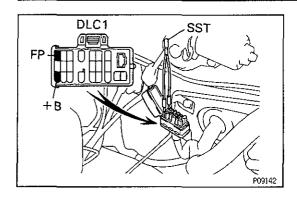
(f) Using SST, connect terminals +B and FP of the check connector.
