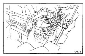
(c) Remove the bolt and distributor.
