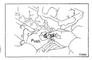
(d) Push the tensioner by hand until it touches the head installation surface, then install the two nuts.
