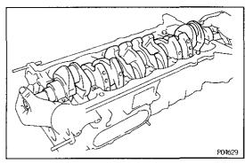
(c) Lift out the crankshaft.
