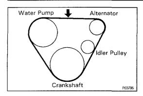
(b) Check the drive belt deflection by pressing on the belt at the points indicated in the illustration with 98 N (10 kgf, 22 lbf) of pressure.
