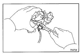
16. REMOVE FUEL CUT SOLENOID VALVE Remove the solenoid valve and gasket.
