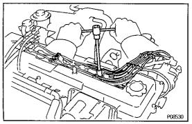
(b) Install the No.1 and No.2 cord clamps with the two bolts.
