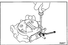
18. REMOVE FAST IDLE CAM BREAKER (FICB) LINK Remove the screw and FICB link.
