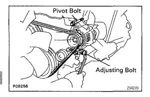
(e) Install the drive belts with the adjusting bolt and pivot bolt.
