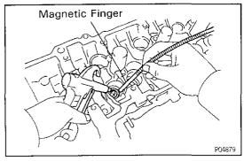
(d) Using compressed air and a magnetic finger, remove the spring seat by blowing air.
