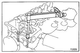
(g) Install and torque the two mounting bolts.
