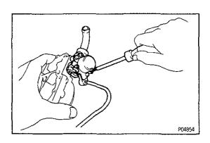
12. REMOVE OUTER VENT CONTROL VALVE (OVCV)
