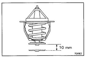
(c) Check the valve lift.
