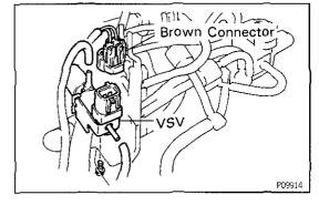
(c) Disconnect the connector and two vacuum hoses, and remove the screw and VSV.
