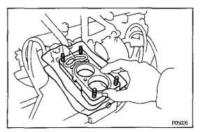
(c) Cover the inlet hole of the intake manifold with a cloth.
