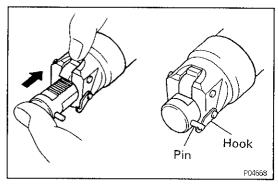
(b) Release the ratchet pawl, fully push in the plunger and apply the hook to the pin so that the plunger cannot spring out.
