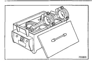
(b) Gradually heat the piston to  $80 - 90^{\circ}\text{C}$  (176 - 194° F).
