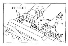
(b) Disconnect the high – tension cords at the rubber boot.
