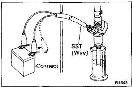
(i) Connect SST (wire) to the injector and battery for 15 seconds, and measure the injection volume with a graduated cylinder. Test each injector two or three times.
