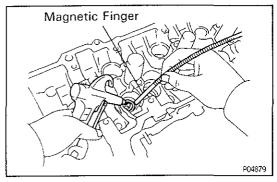
(d) Using compressed air and magnetic finger, remove the spring seat by blowing air.
