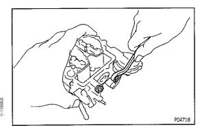
(b) Install the primary and secondary passage plugs with new gaskets.
