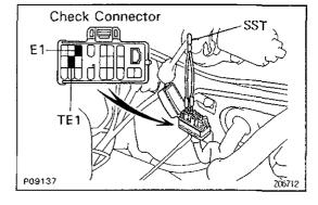
3. Using SST, connect terminals TE1 and E1 of the check connector.
