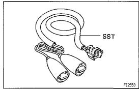
Use SST for inspection or test of the injector or its wiring connector. SST 09842-30070
