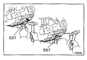
(b) Insert the blade of SST between the No.1 and No.2 oil pans, cut off applied sealer and remove the No.2 oil pan.
