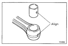
(b) Align the oil holes of a new bushing and the connecting rod.
