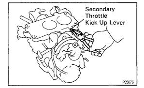
(b) Adjust by bending the secondary throttle kick-up lever.
