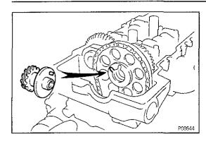
(b) Align the straight pin of distributor gear with the straight pin groove of the intake camshaft gear as shown.
