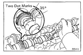
(c) Set the timing mark (two dot marks) of the camshaft driven gear at approx. 35° angle by turning the hexagon wrench head portion of the intake camshaft with a wrench.
