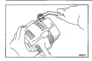
(b) Install the terminal insulator with the nut.
