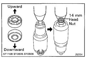
(b) Using a 14 mm head nut and press, press in a new bearing.
