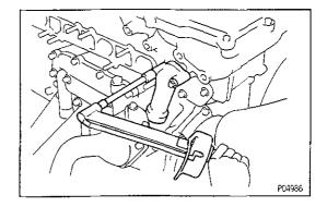
(e) Install the water by—pass outlet and pipe with the two bolts.
