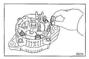
(b) Install the four rubber insulators on the lead wires.
