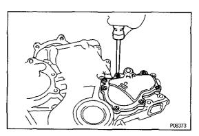
(c) Install the pump cover with the seven screws.
