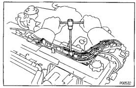
(g) Install the No. 1 and No. 2 cord clamps with two mounting bolts.
