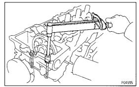
(g) Install and torque the two mounting bolts.
