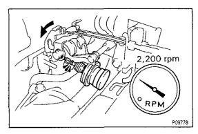
(b) Release the throttle valve gradually, and check the dashpot setting speed when the throttle lever touched the dashpot end.
