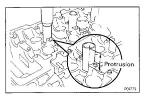
(c) Using a press, press in a new spark plug tube until there is 45.5 mm (1.791 in.) protruding from the camshaft bearing cap installation surface of the cylinder head.
