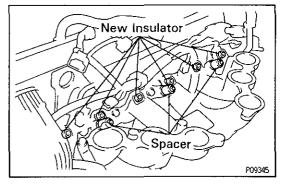
(e) Place six new insulators and the three spacers in position on the intake manifold.
