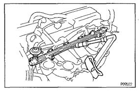
(j) Tighten the three bolts holding the delivery pipe to the intake manifold.
