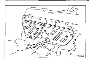
(b) Install the No.1 heat insulator and No.2 heat insulator with the six bolts.
