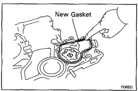
(b) Place a new gasket on the pump body.
