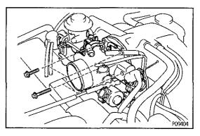
(d) Install the throttle body with the four bolts.
