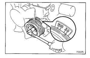
(b) Turn the crankshaft pulley one revolution (360°) and align the its groove with timing mark "0" of the timing chain cover.
