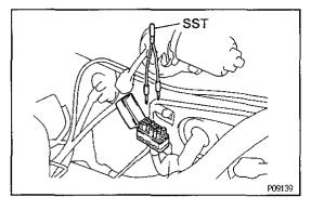
(e) Remove SST from the check connector. SST 09843-18020
