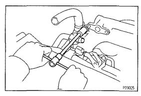
4. REMOVE BOLT HOLDING HEATER INLET PIPE AND AIR INTAKE CHAMBER
