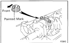
(c) Mark the front of the connecting rod cap nut and bolt with paint.
