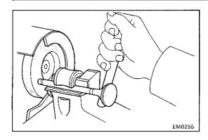
(e) Check the surface of the valve stem tip for wear.
