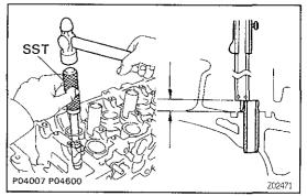
Using SST and a hammer, tap in a new guide bushing (f) to where there 8.2 - 8.6 mm (0.323 - 0.339 in.)protruding from the cylinder head.
