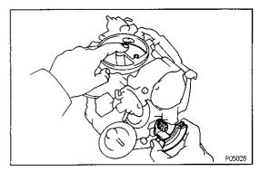
7. CHECK AND ADJUST FAST IDLE CAM BREAKER (FICB)
