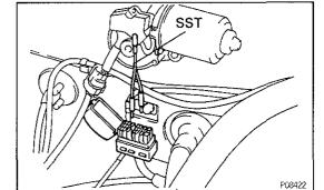
(e) Remove SST from the data link connector 1. SST 09843-18020
