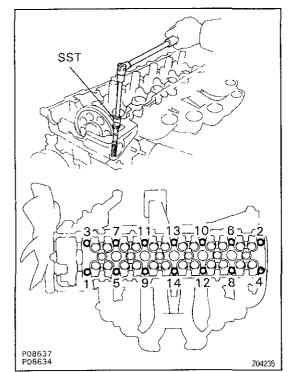
(b) Using SST, uniformly loosen and remove the 14 cylinder head bolts in several passes, in the sequence shown.
