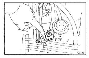
(b) If you have no sound scope, you can check the injector transmission operation with your finger.
