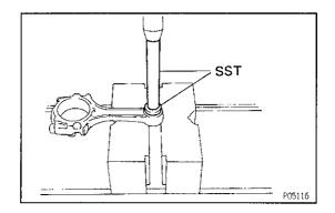
C. If necessary, replace connecting rod bushing
