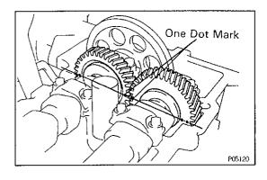
(b) Check that the timing marks (one and two dots) of the camshaft drive and driven gears are in straight line on the cylinder head surface as shown in the illustration. If not, turn the crankshaft one revolution (360°) and align the marks as above.
