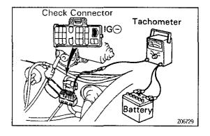
With a tachometer connected to the system, connect the test probe of the tachometer to the IG
