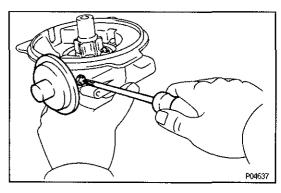
(b) Remove the screw and pull out the vacuum advancer.
