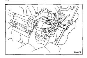
If necessary, loosen the distributor bolt and turn the distributor to align the marks. Recheck the timing after tightening the distributor bolt.
