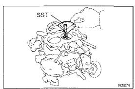
(c) Check the primary throttle valve angle. Standard angle:
