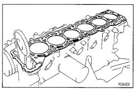
(b) Place a new cylinder head gasket in position on the cylinder block.
