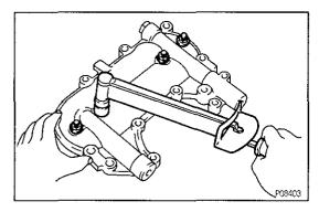
2. ASSEMBLE OIL COOLER AND OIL COOLER COVER
