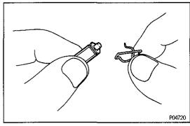
(h) Assemble the clip onto the needle valve.
