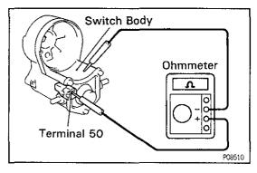
2. PERFORM HOLD—IN COIL OPEN CIRCUIT TEST
