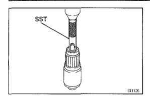
(b) Using SST and a press, press in a new bearing. SST 09201-41020
