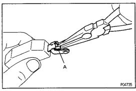
(d) Adjust by bending the portion of the float lip marked A.
