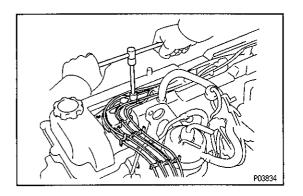
(b) Install the No.1 cord clamp with the bolt.
