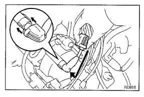
(b) Align the spline of the distributor (ignition coil) with the spline of the holder, and slide on the holder.
