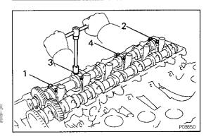
(f) Loosen and remove the No.2, No.3, No.5 and No.7 bearing cap bolts, alternately loosening the left and right bolts uniformly in several passes, in the sequence shown.
