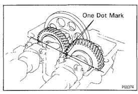
(b) Turn the camshafts so that the timing marks with one and two dots will be in straight line on the cylinder head surface as shown in the illustration.
