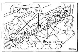
(k) Connect the six injector connectors as shown.
