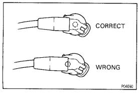
NOTICE: Check that the holder is corretly installed to the grommet and distributor cap as shown in the illustration.
