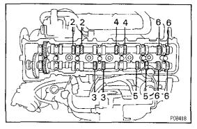
(c) Check only the valves indicated as shown. Measure the valve clearance. (See procedure in step (a))
