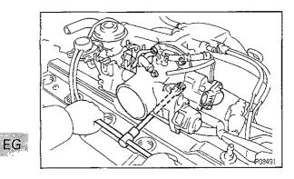
(b) Install a new gasket and throttle body with the four bolts.
