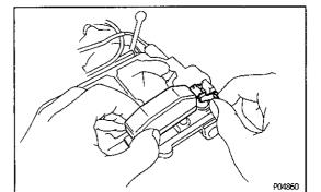
(b) Install the float with the pivot pin.
