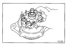
7. REMOVE ROTOR FROM DRIVE END FRAME
