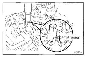
(c) Using a press, press in a new spark plug tube until there is 45.5 mm (1.791 in.) protruding from the camshaft bearing cap installation surface of the cylinder head.
