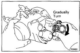
(e) Gradually turn the TP sensor clockwise until the ohmmeter deflects, and secure it with the two set screws.
