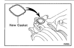
(c) Install a new gasket in position.
