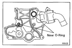
(c) Place two new O-ring in position on the oil pump.
