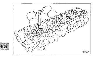
(f) Alternately and uniformly loosen and remove the No.2 and No.5 bearing cap bolts.
