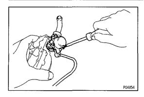
7. INSTALL OUTER VENT CONTROL VALVE (OVCV) Install a new gasket, the wire clamp and OVCV with the three screws.
