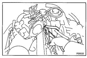
(c) Connect the No.1 water by—pass hose to the throttle body.
