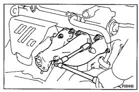
(b) Remove the six nuts, exhaust manifold and gasket.
