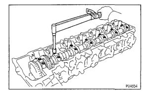
(j) Uniformly tighten the fourteen bearing cap bolts in several passes.
