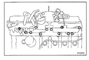
(b) Install the intake manifold and ground strap with the six bolts and two nuts.
