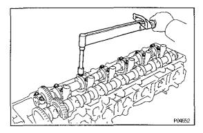
(I) Uniformly tighten the fourteen bearing cap bolts in several passes.
