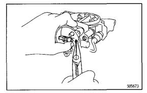
(b) Remove the E-ring, stopper, spring collar and diaphragm.
