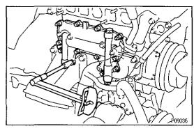
3. INSTALL OIL COOLER AND OIL COOLER COVER ASSEMBLY
