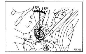
(b) Align the jiggle valve of the thermostat with the protrusion of the water inlet housing, and insert the thermostat in the water inlet housing. HINT: The jiggle valve may be set within 15° of
