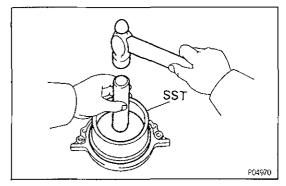
(b) Using SST and a hammer, tap in a new oil seal until its surface is flush with the rear oil seal edge.
