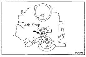
(b) Position the fast idle lever onto the 4th step as shown.
