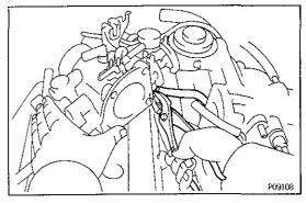
(h) Disconnect the No.1 water by—pass hose from the throttle body, and remove the throttle body.
