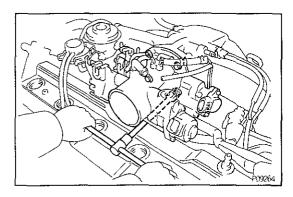
(b) Install a new gasket and throttle body with the four bolts.
