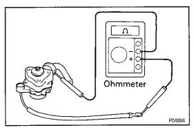
(c) Using an ohmmeter, measure the resistance between the wire terminal and body.
