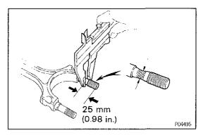
(b) If the cap nut cannot be turned easily, measure the outside diameter of the connecting rod bolt with vernier calipers.
