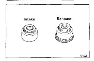
HINT: Different oil seals are used for the intake and exhaust.
