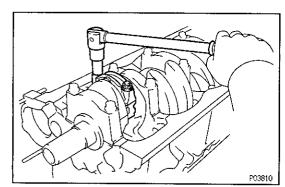
(i) Remove the two nuts and connecting rod cap. (See procedure (b) and (c) above)
