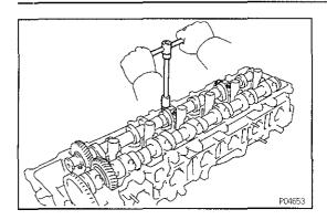
(h) Alternately and uniformly loosen and remove the No.4 and No.6 bearing cap bolts.
