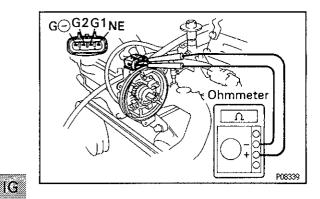
5. INSPECT SIGNAL GENERATOR (PICKUP COIL)
