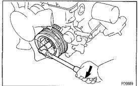
(c) Turn the crankshaft pulley clockwise to provide some slack for the chain on the tensioner side.
