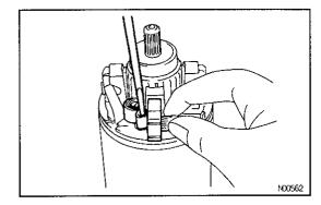
(c) Using a screwdriver, hold the brush spring back, and connect the brush into the brush holder. Connect the four brushes.
