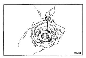
(d) Install the bearing retainer with the four screws.
