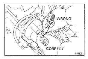
(b) Disconnect the high—tension cord at the grommet. DO NOT pull on the cord. NOTICE:
