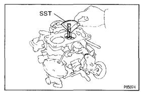
(b) Check the primary throttle valve angle. Standard angle:
