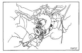
(b) Remove the pivot bolt, lock bolt and alternator.
