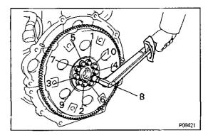
(b) Install and uniformly tighten the ten drive plate bolts in several passes, in the sequence shown.
