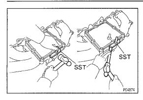
(b) Insert the blade of SST between the intake manifold and water by—pass flange, and cut off applied sealer and remove the flange.
