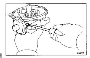
(d) Secure the vacuum advancer with the screw.
