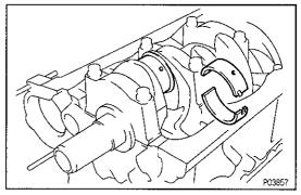
(e) Clean the crank pin and bearing.
