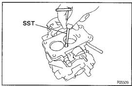
(c) Install the passage screw together with the spring washer.
