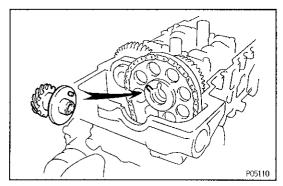
(b) Align the straight pin of distributor gear with the straight pin groove of the intake camshaft gear as shown.
