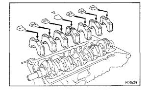
(b) Install the seven main bearing caps in their proper locations.
