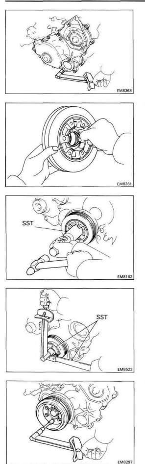
(c) Install the timing gear cover with the fourteen bolts.Torque: 200 kg-cm (14 ft-lb, 20 N⋅m)
