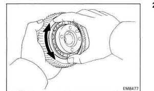
2. **INSPECT INJECTION PUMP DRIVE GEAR BEARING** Check that bearing is not rough or worn.
