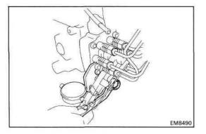
(4) Bolt holding injection pump to injection pump stay.
