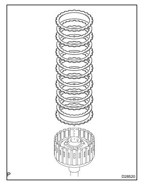
(b) Remove the 2 flanges, the 6 discs and the 5 plates from the input shaft assy.
