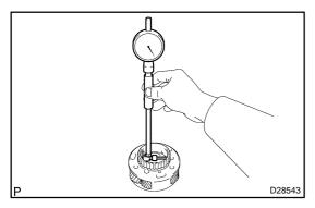
(b) Using a dial indicator, measure the inside diameter of the front planetary gear bushing.
