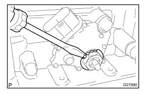
(e) Using a screwdriver, bend the tabs of the lock washer. HINT:
