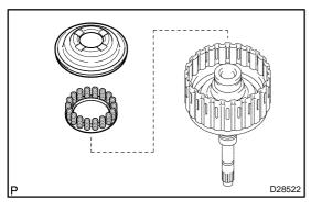
(b) Remove the clutch balancer No.1 and the forwerd clutch return spring from the inputshaft assy.
