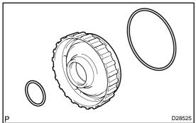
(b) Remove the 2 O-rings from the forward clutch piston.
