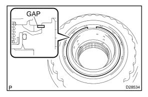
(d) Set the end gap of the snap ring in the piston as shown in the illustration.
