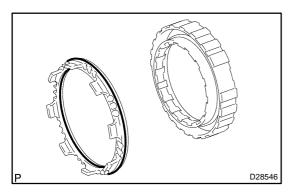
(c) Remove the 2 O-rings from the 2nd brake piston.
