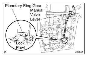
Shift the manual valve lever to the P position, and confirm (b) the planetary ring gear is correctly locked up by the lock pawl.
