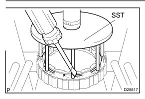
(c) Using SST and press, Install the snap ring. SST 09351-40010
