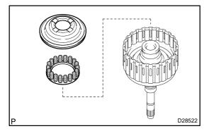
(b) Install the clutch balancer No.1 and the forward clutch return spring sub assy.
