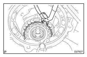
(b) Using SST, install the snap ring. 09350-30020 (09350-07050, 09350-07060) SST
