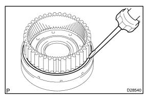
(b) Using a screwdriver, Install the snap ring.
