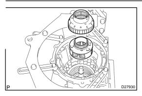
(c) Install the front planetary gear assy and the 1 way clutch inner race from the case.
