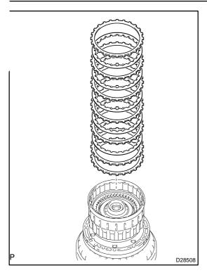
(b) Remove the reverse clutch flange, the 6 plates and the 5 discs from the clutch drum assy.
