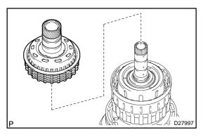
(b) Remove the reverse clutch hub sub assy, the reverse clutch reaction sleeve, the clutch cushion, the plate reverse clutch flange, the 5 reverse clutch discs, and the 4 clutch plates from the clutch drum assy.
