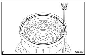
(b) Using a screwdriver, install the hole snap ring.
