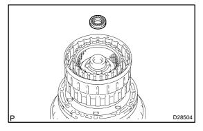
Thrust needle roller bearing diameter: mm (in.)
