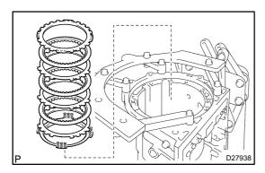
(b) Remove the flange, the brake piston return spring, the 3 discs and the 3 plates from the case.
