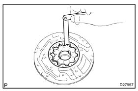
(c) Using a feeler gauge, measure the clearance between the driven gear teeth and the drive gear teeth.
