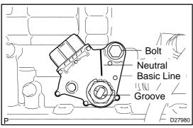
(d) Align the neutral basic line with the switch groove as shown in the illustration, and tighten the adjusting bolt.
