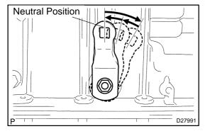
(c) Using the control shaft lever, fully turn the manual lever shaft back and then return 2 notches. It is now in neutral.
