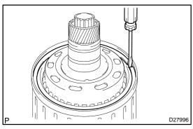
(b) Using a screwdriver, install the snap ring on the clutch drum and the input shaft assy.
