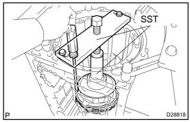
(b) Using SST and press, install the brake No.2 spring snap ring.
