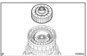
(b) Install the multiple disc clutch clutch hub to the clutch drum assy.
