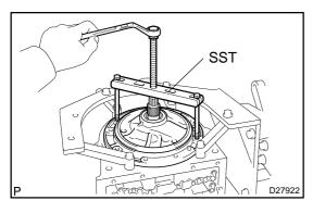
(b) Using SST, remove the oil pump. SST 09350-30020 (09350-07020)
