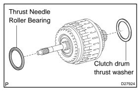
(b) Remove the clutch drum thrust washer and the thrust needle roller bearing.
