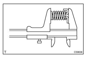
25. INSPECT DIRECT CLUTCH RETURN SPRING SUB-ASSY
