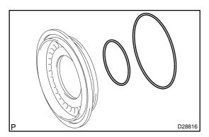
(e) Remove the 2 O-rings from the direct clutch piston Sub-Assy.
