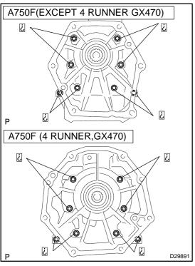
(b) Install the transmission case adapter adapter sub assy with the 8 bolts.
