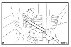
(b) Using feeler gauge, measure the B3 brake pack clearance between the snap ring and the flange.
