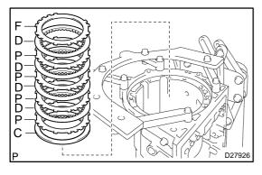
(a) Install the 2 flanges, the 4 discs and the 4 plates on the case.
