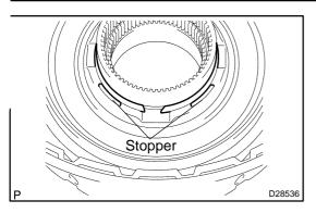
(g) Set the end gap of the snap ring in the piston as shown in the illustration.
