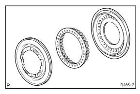
(b) Install the clutch balancer No.2 and the direct clutch return spring to the direct clutch piston sub assy.
