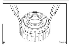
(b) Using 2 screw drivers, remove the direct clutch piston sub assy from the clutch drum.
