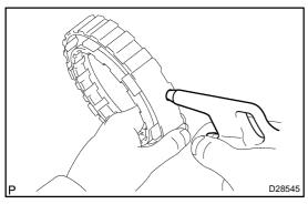
(b) Hold the 2nd brake piston and apply compressed air (392 kPa, 4.0 kgf/cm², 57 psi) to the 2nd brake cylinder to remove the 2nd brake piston.
