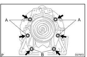
(d) Install the gasket from the extension housing.
