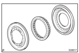
(d) Remove the clutch balancer No.2 and the direct clutch return spring sub assy from the direct clutch piston sub assy.
