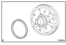
(c) Remove the thrust bearing race No.1 from the front oil pump.
