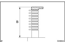
(c) Using vernier calipers, measure the thickness (length B) of the 2 brake flanges, the 7 brake plates No.4 and the 8 brake discs No.4 altogether at the both end across a diameter, and calculate the average.
