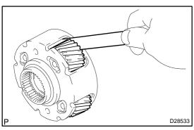
60. INSPECT CTR PLANETARY GEAR ASSY
