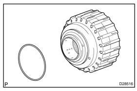
(c) Remove the O-ring from the clutch drum.
