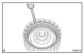
(b) Using a screwdriver, install the hole snap ring.
