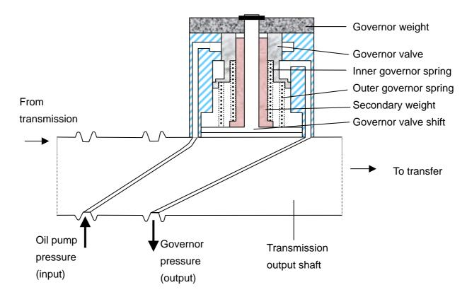
As the vehicle speed increases, the centrifugal force of the weights also increases, hence the greater governor pressure necessary to balance the centrifugal force. Eventually, vehicle speed reaches a point at which the governor valve cannot balance itself against the centrifugal force of the weight. The governor valve is permanently in the open position and governor pressure equals the mainline supply pressure.
