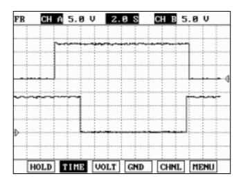
1) Measure the output signal of SCSV 1 & 2 (CH-A: SCSV1, CH-B: SCSV2)
