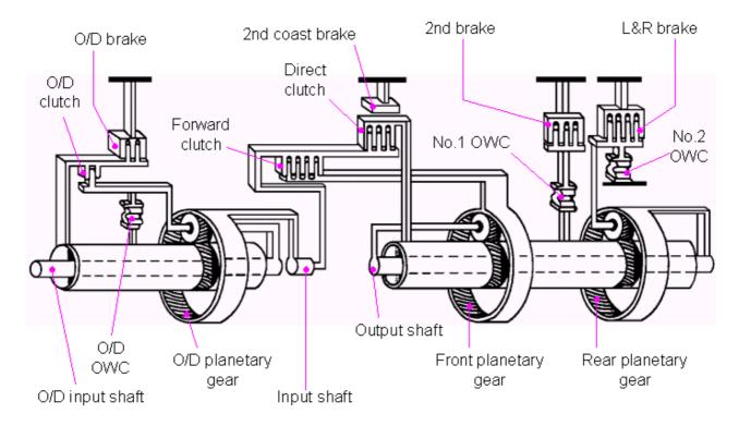
C0: O/D clutch - Connects O/D sun gear and O/D carrier
