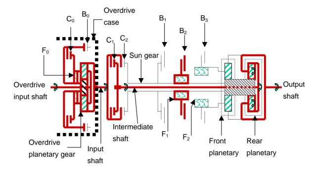
\*B1 applies (when engine braking is applied at "2" range
