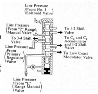
\* At 'L' range, the spool moves upward because the line pressure from a manual valve applies to 'B': 3<sup>rd</sup> gear is impossible
