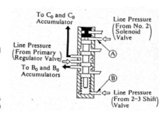
\* At '2', 'L' range, the spool moves upward because the line pressure from a 2-3 shift valve applies to 'B': 4<sup>th</sup> gear is impossible
