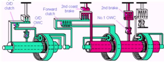
No.1 OWC is always engaged due to the 2nd coast brake regardless of vehicle acceleration or deceleration. → Engine brake is available.
