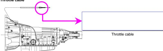
Due to the line not pressure control by solenoid valve but the throttle cable controls pressure, it is very important to adjust correctly the throttle cable between A/T and fuel injection pump.
