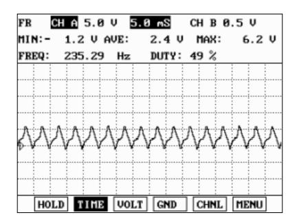
1) Measure the waveform of PG-A in 3<sup>rd</sup> gear.
