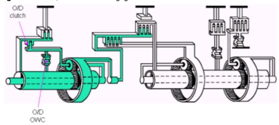
'R' range - O/D clutch, O/D OWC, Direct clutch, L&R brake are engaged.
