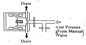
\* Sol. Type: NC (Normal close): When ON, it is open → line pressure to shift valve drains
