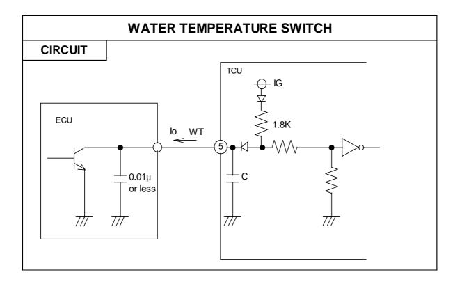
Io: 10mA max. (at IG = 16V) Leak resistance: 100K·min. Chattering time: 10msec. Max.
