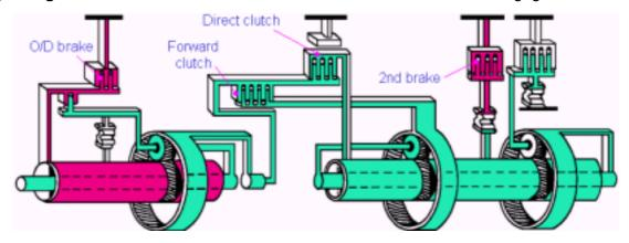
**'2' or 'L' range 2nd gear** - O/D clutch, O/D OWC, Forward clutch, 2nd brake, 2nd coast brake, No.1 OWC are engaged.
