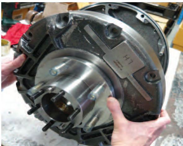
Figure 138: Slide housings together using the alignment dowels to assist.
