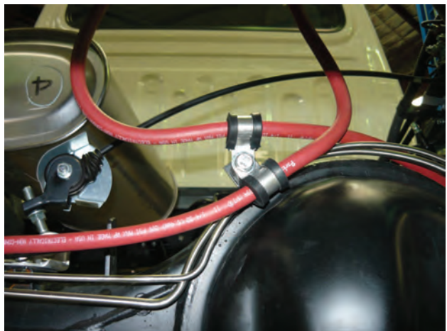
Figure 39: Breather routing at rear differential.
