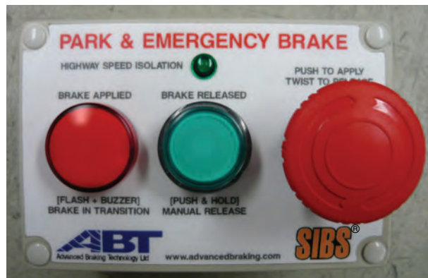
Figure 114: Control box fascia
