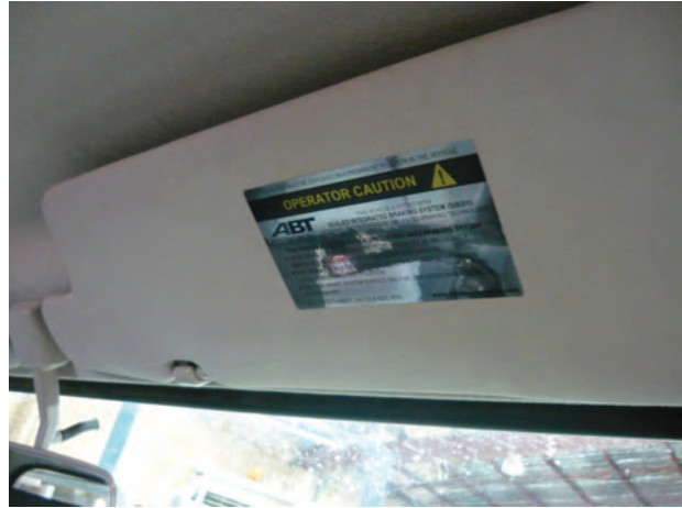
Figure 120: “Operator Caution” label on driver’s sun visor.
