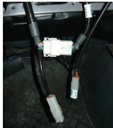
Figure 77: Connect the 12 pin Cabin Control harness within the glove box.
