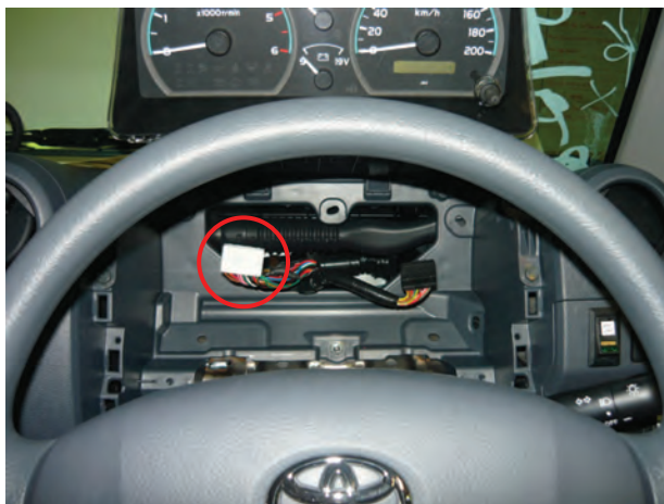
Figure 83: Take the LH multi-plug.
