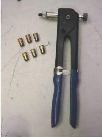
Figure 9: Insertion Tool and M8 Inserts Front brakes only – Textron P/N; 39006-28035
