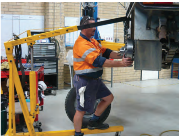
Figure 22: Fitting the housing & hub complete
