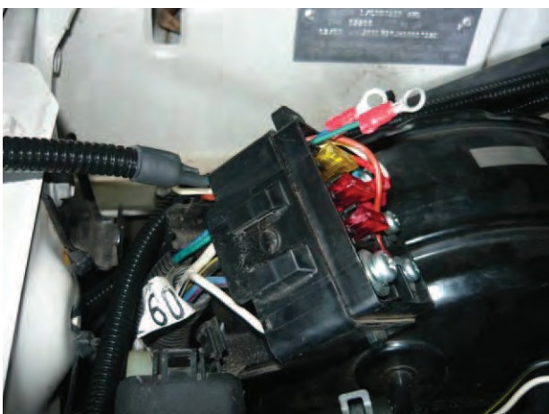
Figure 89: Fit the SIBS ® power cables into the Toyota power outlet box.
