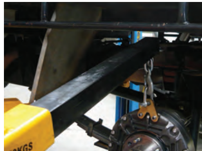
Figure 20: Housing fitted complete with hub using lifting hoist and lifting eye.
