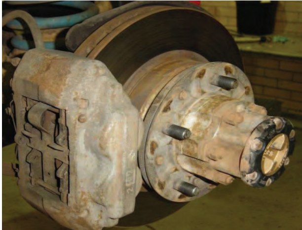
Figure 3: Conventional OE dry disc and rotor
