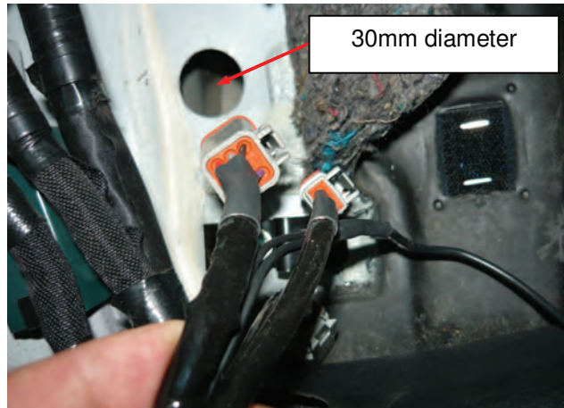
Figure 58: Feed plugs through the bulkhead
