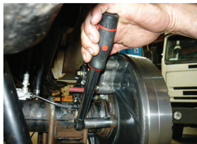
Figure 23: Secure the SIBS ® II housing (81Nm)
