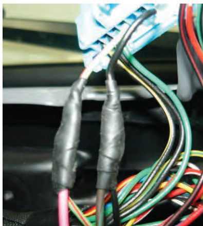
Figure 76: Use self-amalgamating insulation tape to seal the joint.
