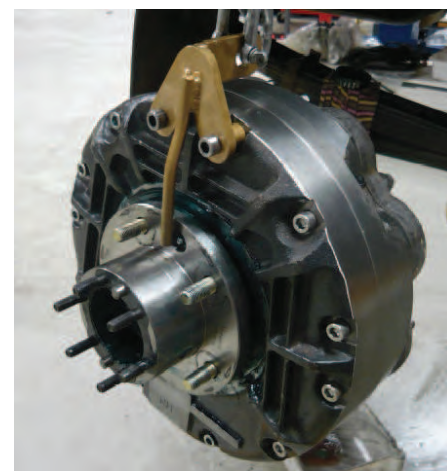
Figure 139: Install the lifting eye (P/N; 24-2870) in place of the top two housing bolts.
