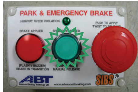
Figure 95: Brake RELEASED indication
