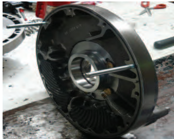
Figure 135: Fit the alignment dowels (P/N; 24-2883)
