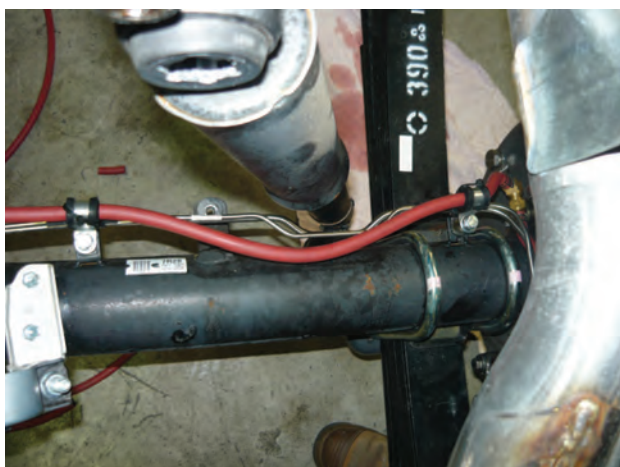
Figure 38: Avoid hose contact with LH damper.
