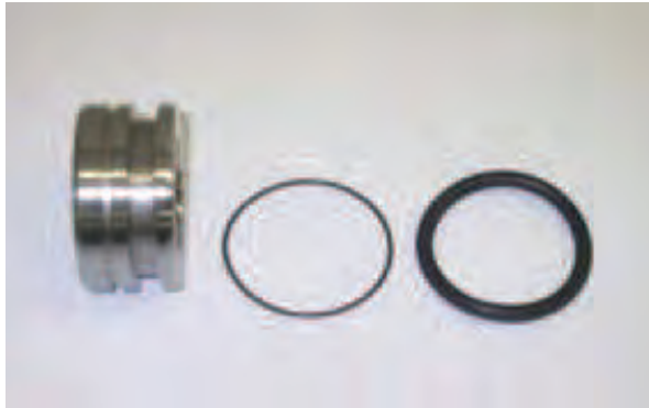
Figure 129: Service piston, EPDM O-ring (large) and Viton Wiper O-ring (small)
