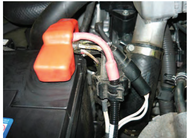
Figure 92: Main power cable securely clipped to OE Toyota harness.
