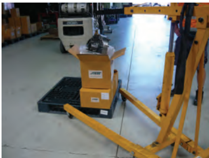
Figure 19: SIBS ® II assembly being removed from box using hoist and lifting eye
