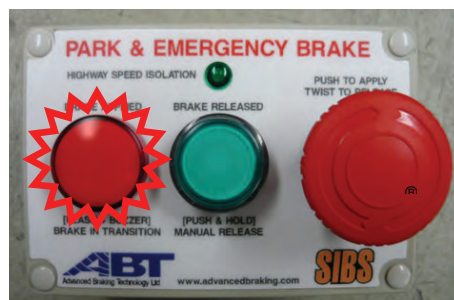
Figure 97: Brake APPLIED indication
