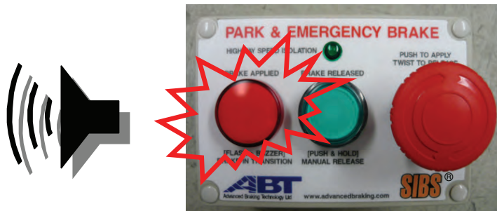
Figure 96: Brake TRANSITION indication
