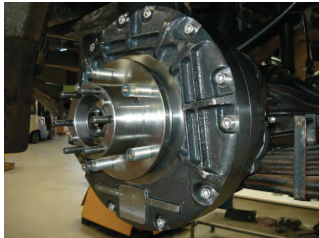
Figure 4: SIBS ® II fully sealed wet brake
