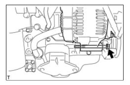
(c) Remove the bolt and generator w/ vacuum pump assembly.
