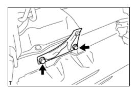
(a) Remove the 2 bolts and intake air connector bracket.
