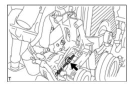
(b) Remove the bolt and spacer.
