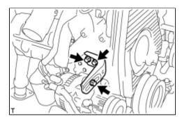
(a) Remove the 3 bolts and fan belt adjusting bar.
