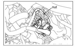
(e) Remove the connector and nut, as shown the illustration.
