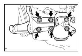
(a) Remove the 6 bolts and pump bracket.
