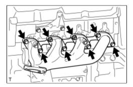
(a) Remove the 6 bolts, 2 nuts and exhaust manifold.
