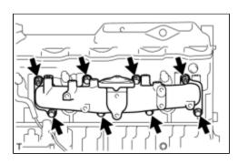
(a) Remove the 6 bolts, 2 nuts, intake manifold and gasket.
