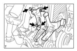
(c) Remove the 4 bolts and compressor mounting bracket.
