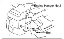
(a) Install the engine hanger No.2 in the correct direction.
