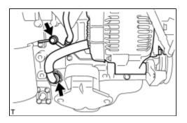
(a) Remove the bolt with the hose disconnected.
