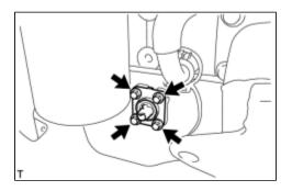
(a) Remove the 4 bolts and engine oil level sensor.
