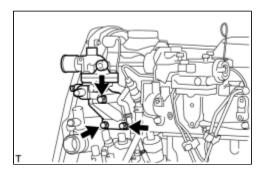
(a) Remove the 3 bolts, water outlet, outlet housing assembly and gasket.
