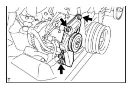
(a) Remove the 3 bolts and compressor mounting bracket.
