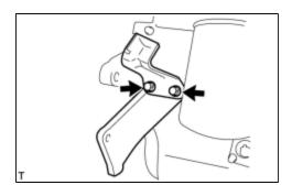
(a) Remove the 2 bolts, exhaust pipe support bracket No.1 and stiffener plate RH.
