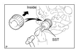
(a) Align the pulley set key with the key groove of the timing pulley.
