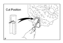
(a) Using a knife, cut off the oil seal lip.
