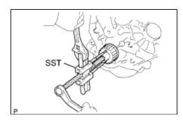
(a) Remove the crankshaft timing pulley.
