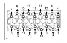
(a) Uniformly loosen and remove the 18 cylinder head bolts, in several steps, in the sequence shown.
