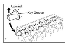
(1) Place the camshaft on the cylinder head with the key groove facing upward.
