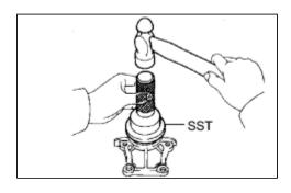
(a) Using SST and a hammer, tap in a new oil seal until its surface is flush with the oil seal retainer edge.
