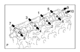
(3) Apply a light coat of engine oil to the threads and under the heads of the bearing cap bolts.
