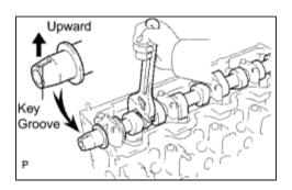
(a) Turn the camshaft with a wrench so that the key groove faces upward.
