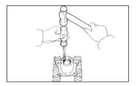
(a) Using a screwdriver and hammer, tap out the oil seal.
