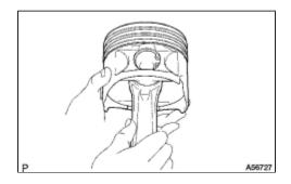
(1) Try to move the piston back and forth on the piston pin.
