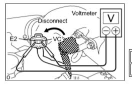
(3) Using a voltmeter, measure the voltage according to the value(s) in the table below.
