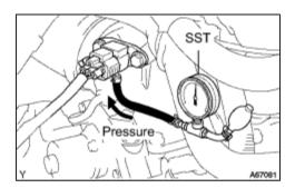
(6) Using SST (turbocharger pressure gauge), apply pressure to the sensor, from 19.69 kPa (0.20 kgf\*cm, 2.84 psi) to 98.0 kPa (1.0 kgf\*cm, 14.2 psi) in steps.
