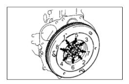
(e) Install and uniformly tighten the 8 bolts in several steps, in the sequence shown.
