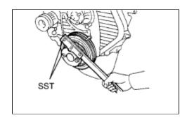
(a) Using SST, hold the crankshaft.
