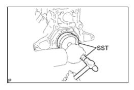
(a) Apply MP grease to a new oil seal lip.
