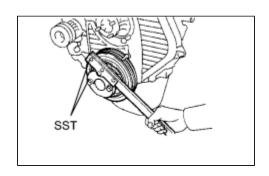
(a) Fix the crankshaft with SST, then remove the 8 bolts and flywheel.
