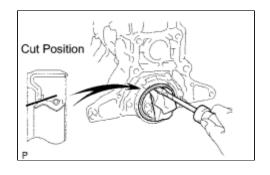
(a) Using a knife, cut off the oil seal lip.
