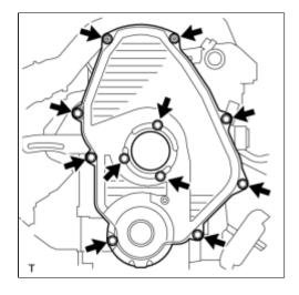
(c) Install the timing belt cover with the 11 bolts.
