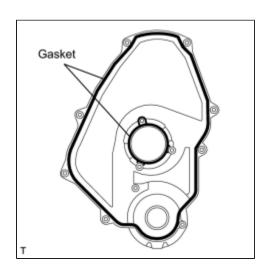
(b) Install the 2 gaskets to the timing belt cover.
