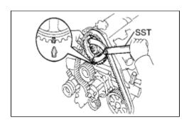
clockwise. Hang the timing belt on the timing pulley, and align the timing marks of the timing pulley and timing belt case.
