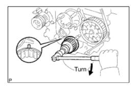
(a) Using the crankshaft pulley bolt, align its groove with the timing pointer by turning the crankshaft clockwise.
