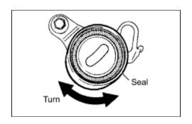
(a) Visually check the seal portion of the timing belt idler No.1 for oil leakage.
