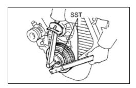
(b) Using SST, install the pulley bolt.
