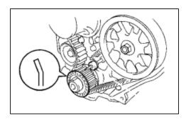
(a) Install the belt guide with the cup side facing outward.
