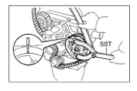
(c) Using SST, slightly turn the injection pump drive pulley clockwise. Hang the timing belt on the pulley, and align the timing marks of the drive pulley and timing belt case.
