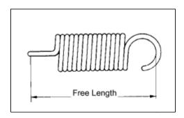
(a) Measure the free length of the tension spring.
