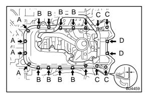
Temporarily install the No.1 oil pan with the 19 bolts, stud bolt and 2 nuts.
