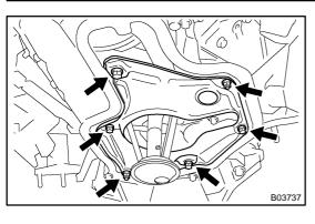
11. REMOVE OIL PAN BAFFLE PLATE
