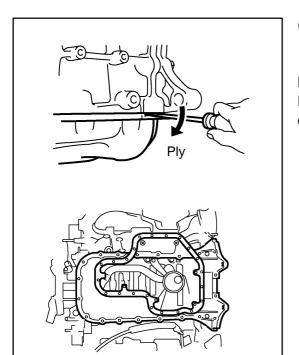
(b) Using a screwdriver, remove the No.1 oil pan by prying between the oil pan and cylinder block in the sequence shown.
