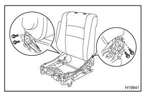
(d) Remove the 4 bolts and seatback assembly. **NOTICE:**
