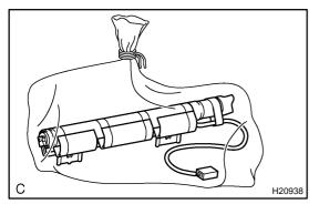
3. DEPLOYMENT WHEN DISPOSING OF CURTAIN SHIELD AIRBAG ASSEMBLY WITH AIRBAG DEPLOYED IN COLLISION
