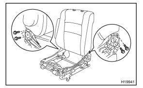
(b) Install the seatback assembly with the 4 bolts. Torque: 43 N-m (440 kgf-cm, 32 ft-lbf)
