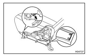
7. **REMOVE LOWER SEAT CUSHION SHIELD** Remove the screw and lower seat cushion shield as shown in the illustration.
