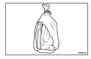
3. DEPLOYMENT WHEN DISPOSING OF SIDE AIRBAG ASSEMBLY WITH AIRBAG DEPLOYED IN COLLISION Dispose of the side airbag assembly.
