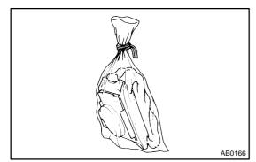
(g) Dispose of the steering wheel pad (with airbag). **CAUTION:**
