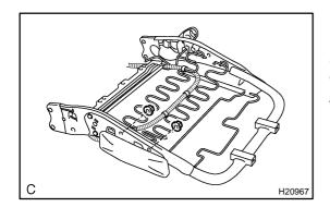
(a) Remove the 2 nuts and side airbag assembly from the seatback assembly, then disengage the clamps.
