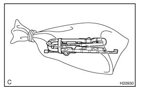
(c) Put the removed curtain shield airbag in a clear plastic bag and keep it in a safe place.
