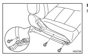
8. **INSTALL LOWER SEAT CUSHION SHIELD** Install the lower seat cushion shield with the screws.
