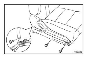
6. **REMOVE SEAT CUSHION INNER SHIELD** Remove the 3 screws and seat cushion inner shield.
