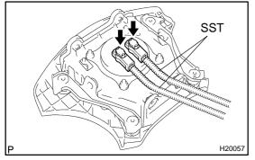
Install the 2 bolts with washers in the 2 bolt holes in the steering wheel pad.
