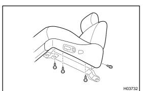
(b) Install the seat cushion outer shield with the 4 screws.11. INSTALL SEATBACK BOARD
