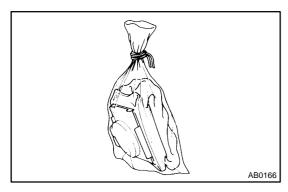
3. DEPLOYMENT WHEN DISPOSING OF STEERING WHEEL PAD WITH AN AIRBAG DEPLOYED IN A COL-LISION
