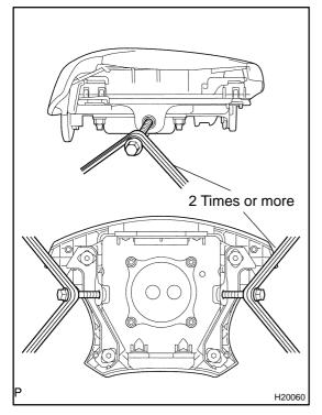
(3) Using 3 wire harness, wind the wire harness at least2 times each around the bolts installed on the leftand right sides of the steering wheel pad.
