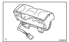
(a) Remove the front passenger airbag assembly (See page RS-31).
