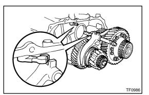
17. REMOVE IDLER GEAR ASSEMBLY WITH CENTER DIFFERENTIAL ASSEMBLY, SHIFT FORK NO. 1 AND SHIFT FORK NO. 1 SHAFT FROM FRONT CASE
