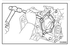
(b) Using a brass bar and hammer, tap the case cover and remove it.
