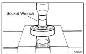
(b) Using a socket wrench and press, remove the rear ball bearing.
