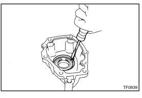
(b) Using SST and a press, remove the ball bearing. SST 09316-6001 1 (09316-00011, 09316-00071)
