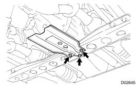
**REMOVE TRANSFER CASE PROTECTOR** 2. Remove the 3 bolts and transfer case protector. Torque: 28 N·m (290 kgf·cm, 21 ft·lbf)
