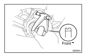
18. INSTALL CLUTCH SLEEVE WITH SHIFT FORK NO. 2 SHAFT AND SHIFT FORK NO. 2
