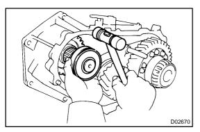
16. REMOVE INPUT SHAFT ASSEMBLY
