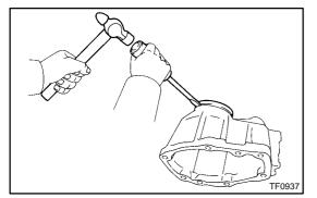
(b) Using a screwdriver and hammer, tap the dust deflector and remove it from the extension housing.
