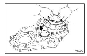
15. REMOVE 2 BEARING RACES FROM REAR CASE
