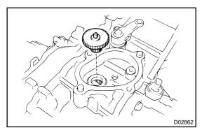
4. REMOVE OUTPUT GEAR FROM FRONT CASE
