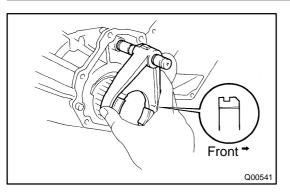
8. REMOVE CLUTCH SLEEVE WITH SHIFT FORK NO. 2 SHAFT AND SHIFT FORK NO. 2
