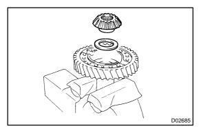
(c) Remove the front side gear and thrust washer.
