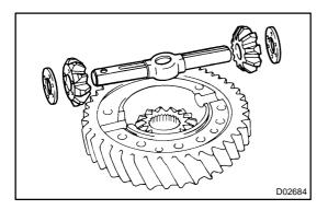
(b) Remove the pinion shaft, 2 pinion gears and thrust washers.
