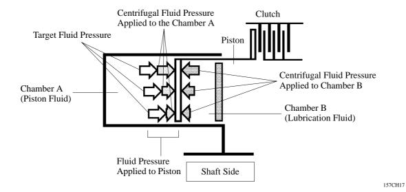
Fluid pressure applied to piston — Centrifugal fluid pressure applied to chamber B = Target fluid pressure (original clutch pressure)
