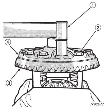
Fig. 50 Ring Gear Bolt Installation
