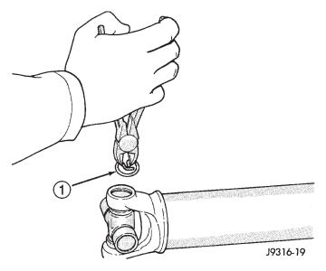
Fig. 18 Remove Snap Ring
