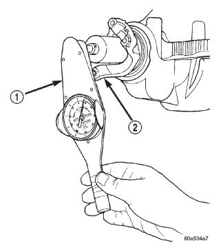
Fig. 48 Check Pinion Rotation Torque
