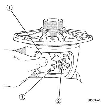
Fig. 52 Pinion Mate Gear Removal
