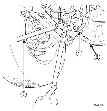
Fig. 47 Tightening Pinion Nut—Typical
