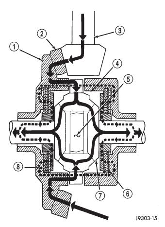
**Fig. 4 Trac-lok** Limited Slip Differential Operation
