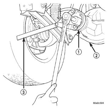
Fig. 16 Tightening Pinion Nut
