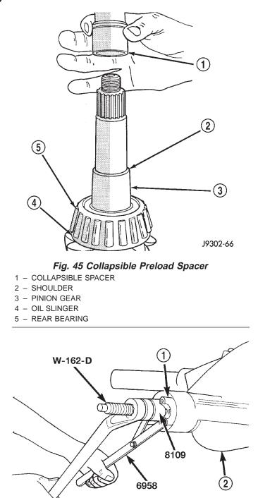
Fig. 46 Pinion Yoke Installation
