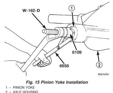
NOTE: If new pinion bearings were installed, do not install the differential assembly and axle shafts until after the pinion bearing preload and rotating torque are set.
