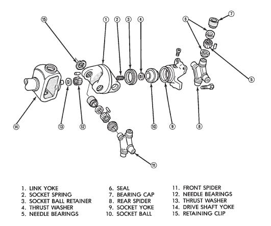
Fig. 4 Double Cardan U-Joint
