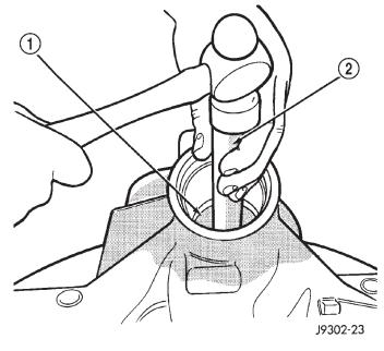
Fig. 38 Rear Bearing Cup Removal
