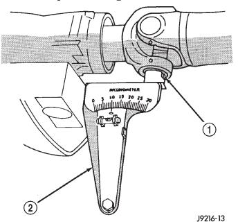
Fig. 9 Front (Output) Angle Measurement (A) 1 – SLIP YOKE BEARING CAP
