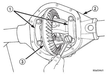
Fig. 62 Tighten Bolts Holding Bearing Caps
