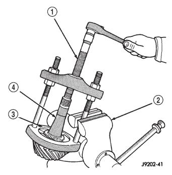
Fig. 40 Inner Bearing Removal
