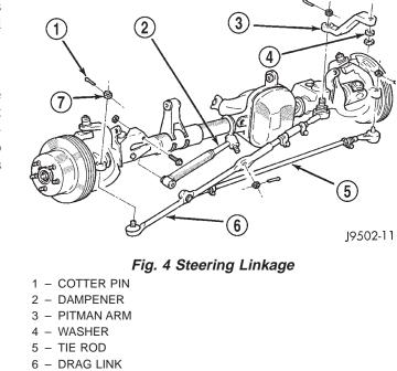
(4) Adjust the left wheel toe position with the tie rod. Turn the sleeve until the left wheel is at the same TOE-IN position as the right wheel. Position the clamp bolts as shown (Fig. 3) and tighten to 27 N·m (20 ft. lbs.). Make sure the toe setting does not change during clamp tightening.
