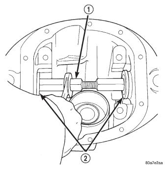
Fig. 33 Axle Seal Installation
