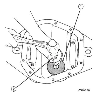
Fig. 41 Rear Pinion Bearing Cup Installation
