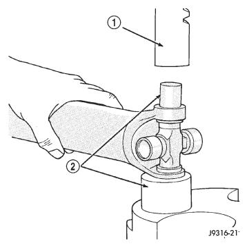
Fig. 19 Press Out Bearing
