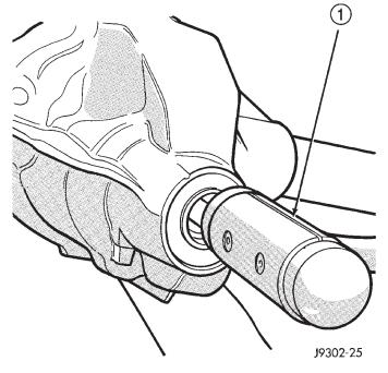
*Fig. 12 Remove Pinion Gear* 1 – RAWHIDE HAMMER
