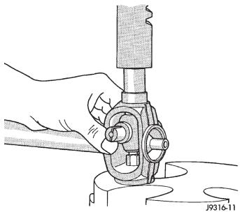
Fig. 29 Press In Bearing Cap
