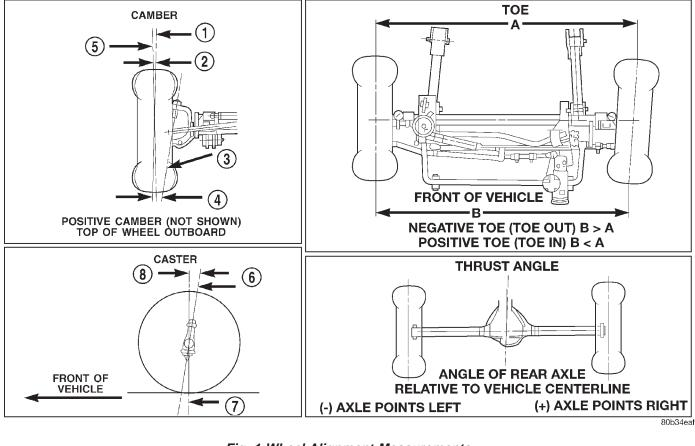
Fig. 1 Wheel Alignment Measurements
