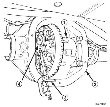
Fig. 65 Differential Side play Measurement
