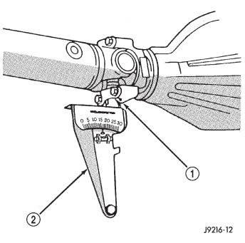
Fig. 11 Rear (Input) Angle Measurement (B)
