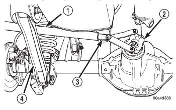
Fig. 34 Pinion Yoke Holder—Typical
