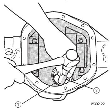
Fig. 37 Front Bearing Cup Removal 1 – REMOVER 2 – HANDLE
