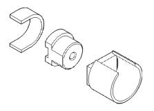
Remover/Installer Suspension Bushing 7932
