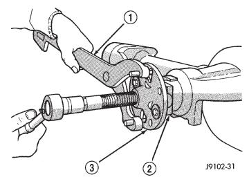
Fig. 35 Pinion Yoke Removal
