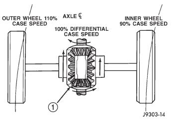
**Fig. 3 Differential Operation—On Turns** 1 – PINION GEARS ROTATE ON PINION SHAFT
