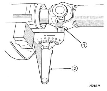
Fig. 10 Propeller Shaft Angle Measurement (C)
