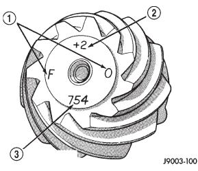
Fig. 55 Pinion Gear ID Numbers
