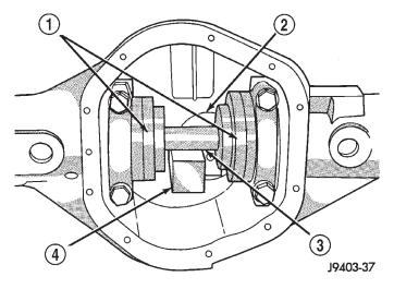
Fig. 59 Gauge Tools In Housing—Typical
