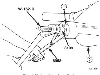
Fig. 8 Pinion Yoke Installation
