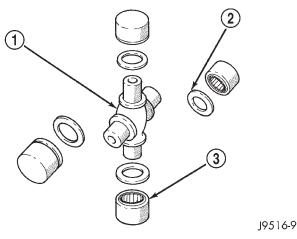
Fig. 3 Single Cardan U-Joint
