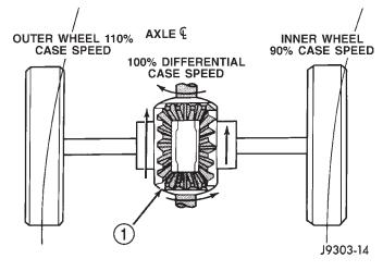
**Fig. 2 Differential Operation—On Turns** 1 – PINION GEARS ROTATE ON PINION SHAFT
