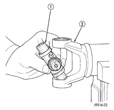
Fig. 21 Install Cross In Yoke
