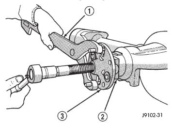
Fig. 11 Pinion Yoke Removal
