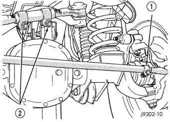
**Fig. 3 Drag Link and Tie Rod Clamp** 1 – TIE ROD CLAMP 2 – DRAG LINK CLAMPS
