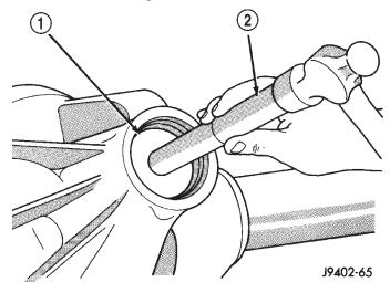
Fig. 42 Pinion Outer Bearing Cup Installation 1 - INSTALLER 2 - HANDLE
