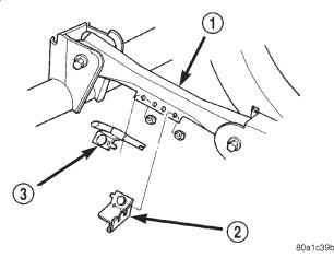
Fig. 4 Parking Brake Cable/Bracket And Wiring Bracket
