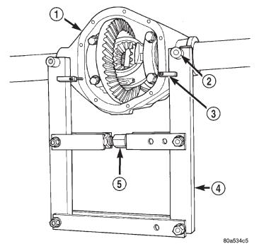
Fig. 25 Install Axle Housing Spreader
