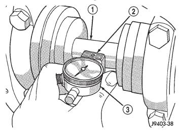
**Fig. 60 Pinion Gear Depth Measurement—Typical** 1 – ARBOR
