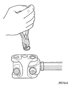
Fig. 23 Remove Snap Rings
