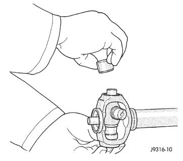
Fig. 28 Install Bearing Cap
