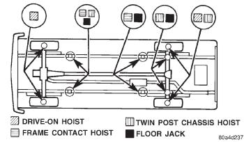
Fig. 6 Vehicle Lifting Locations
