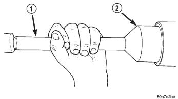
Fig. 43 Pinion Seal Installation
