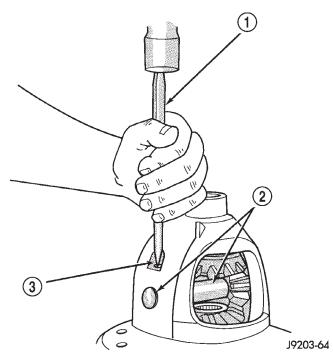
Fig. 53 Mate Shaft Roll Pin Installation
