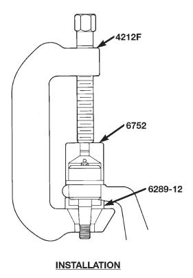
Fig. 22 Upper Ball Stud Remove/Install
