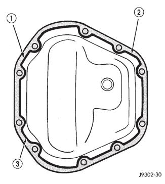
Fig. 3 Typical Housing Cover With Sealant
