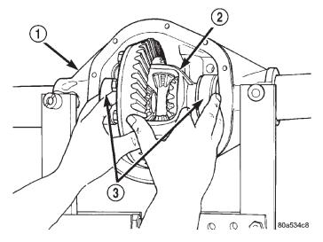
Fig. 28 Differential Case Removal
