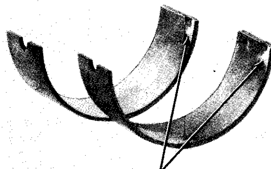
Fig. 1B-92 Scoring Caused by Dirt
