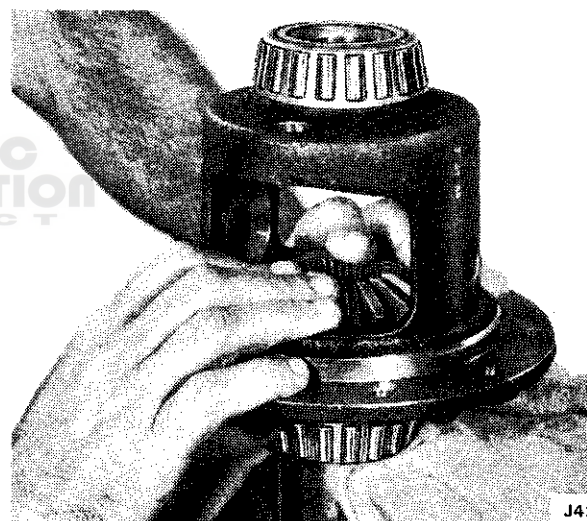
Fig. 2F-70 Remounting Differential Case on Axle Shaft
