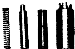
J-21872 PISTON PIN REMOVER AND INSTALLER
