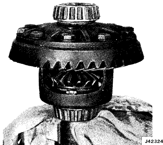
Fig. 2F-62 Differential Mounted on Axle Shaft
