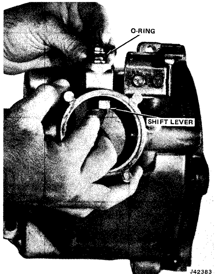
Fig. 2D-37 Shift Lever O-Ring Installation
