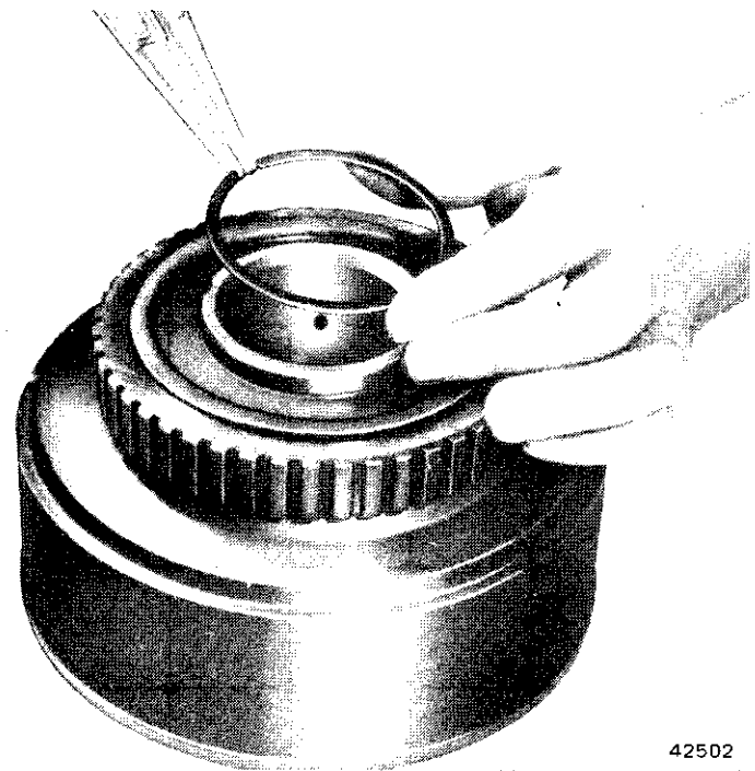
Fig. 2C-84 Intermediate Roller Clutch Snap Ring Removal
