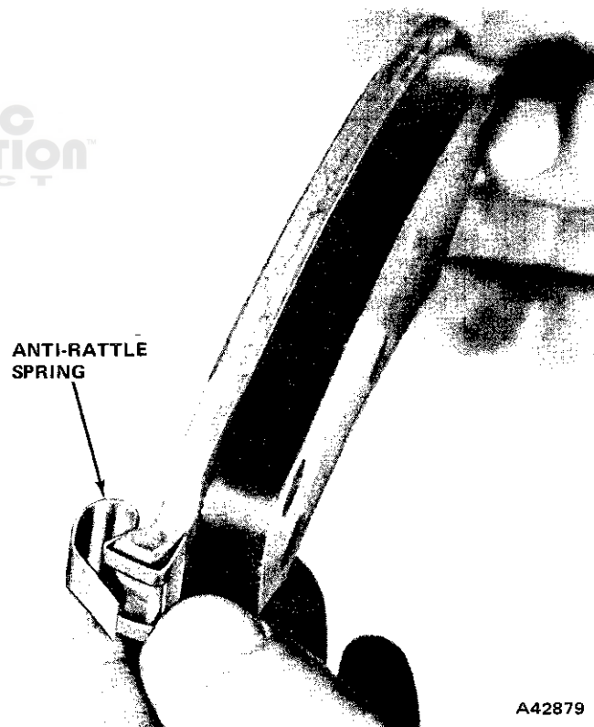
Fig. 2G-48 Installing Anti-Rattle Spring On Inboard Brakeshoe
