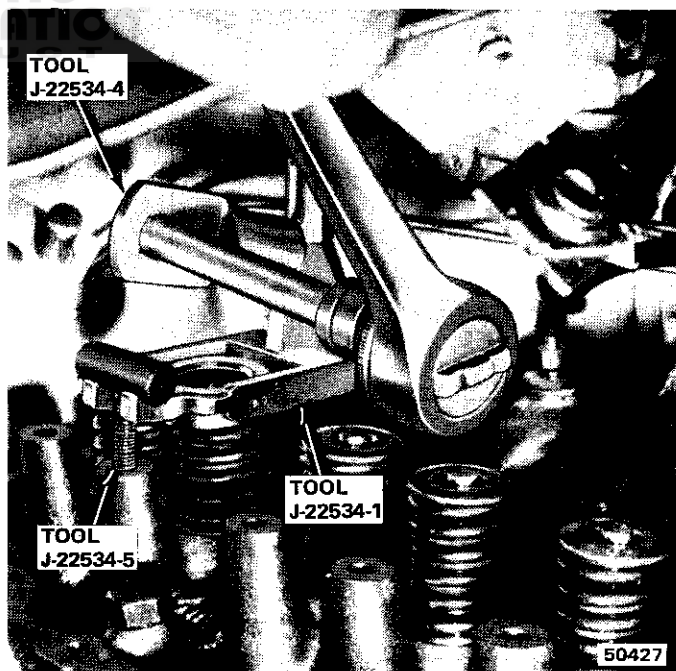
Fig. 1B-12 Valve Spring Removal
