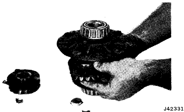
Fig. 2F-68 Side Gear and Clutch Pack Removal
