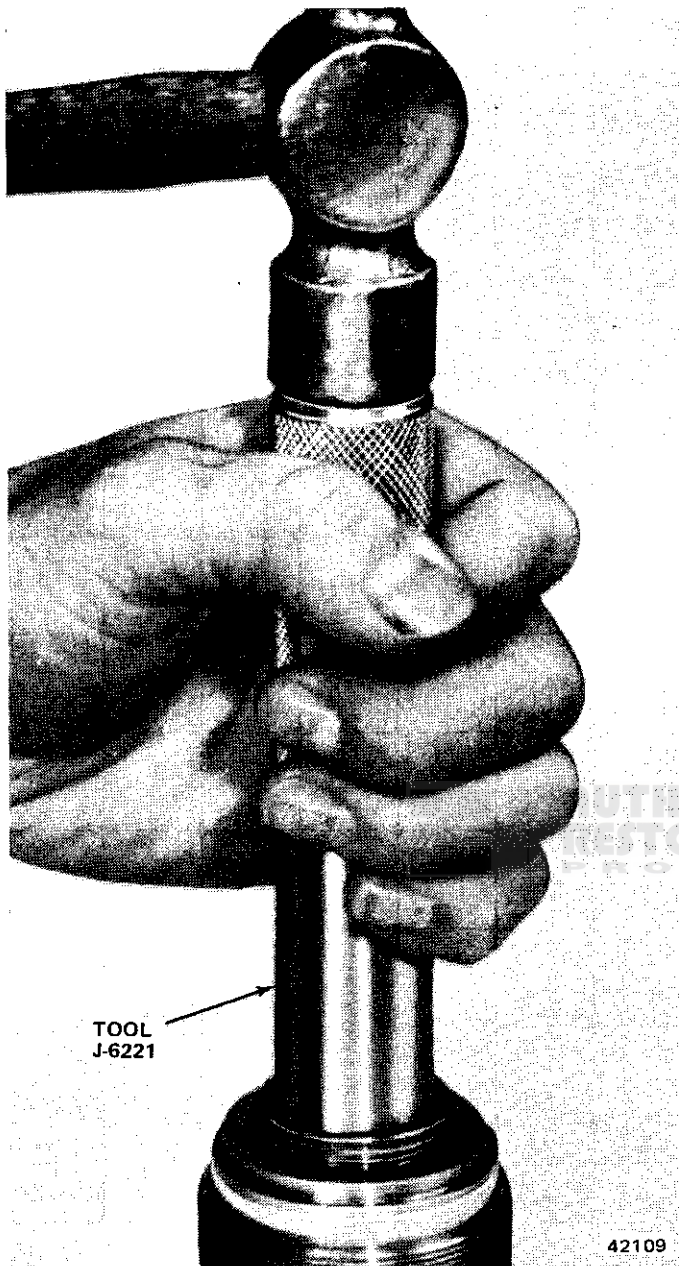
Fig. 2L-25 Adjuster Plug Needle Bearing Removal/Installation
