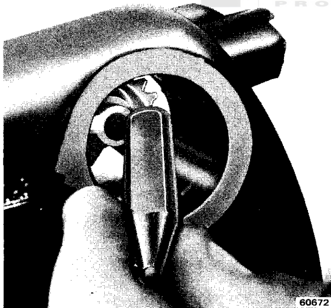
Fig. 2J-17 Sector Installation
