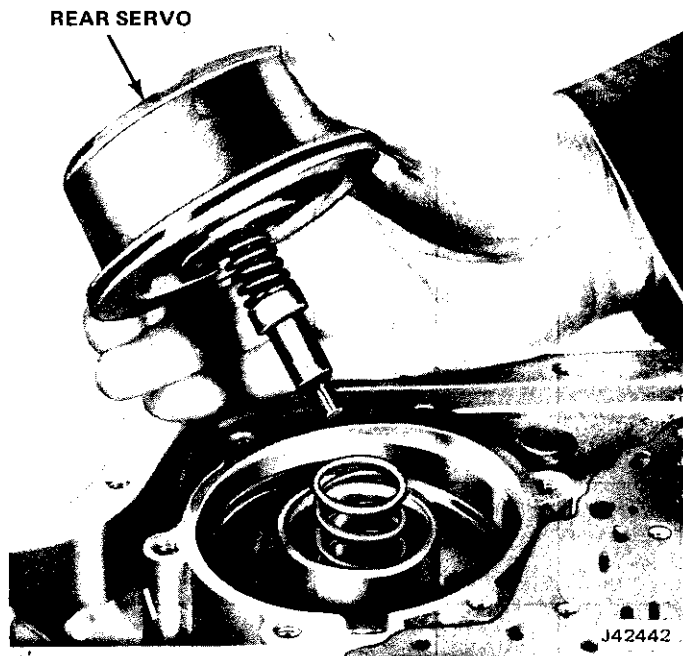
Fig. 2C-19 Rear Servo Removal/Installation
