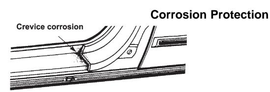
**Crevice corrosion** is a form of localized attack that occurs in areas on metal surfaces exposed to the elements. Examples include spot weld lap joints, threaded or riveted connections, gasket fittings, porous welds, valve seats.
