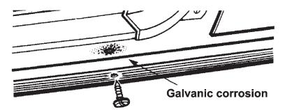
Galvanic corrosion is the type that occurs when dissimilar metals are in electrical contact while immersed in an electrolyte.
