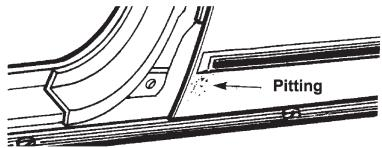
Pitting is the corrosion of a metal surface at points or small areas which look like a small hole in the metal.
