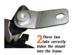
This is the mount bolted to the passenger side shock tower.
