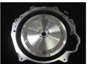
P/N 716131-A Chevy block to Jeep Torqueflite P/N 716131-V Chevy Gen III Vortec V8 block to Jeep Torqueflite (Some 727 transmissions, when coupled to a stock V8, may require a new torque converter)
