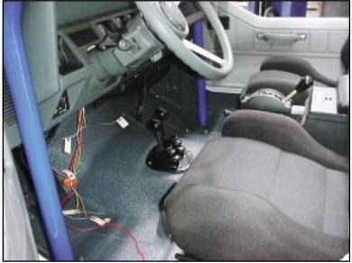
16 This is the correct boot position for the twin sticks. When installing, be sure they do not hit the floor when in full movement.
