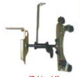
(Brkt. #4) This bracket (used mostly in TJs and some Cherokees) is by far, the hardest linkage to retain when doing any type of conversion. The outside of the bracket is bolted to the frame rail or floorboards, thus causing difficulty adjusting for different transmission lengths.
