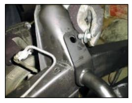
Installation of the upper frame bolt. (Note the removal of the shock to access the nut from the outside.
