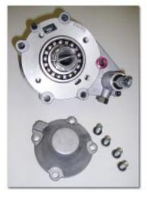
Bearing cap & screws removed. (During the reassembly, the 4-3/8" cap screws should be torqued to 19 ft./lbs., and the 1/4" cap screw to 6 ft./lbs. of torque)
