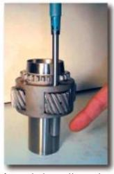
synchro-teeth. To prevent the pin from spinning and/or moving back and forth, we also started putting a small tack weld on the bottom of each pin.
