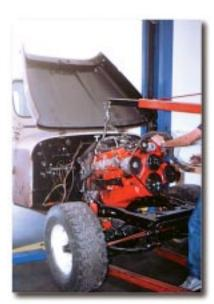
When mounting the block into a Jeep, it is recommended to remove the grille and fenders for ease of installation.
