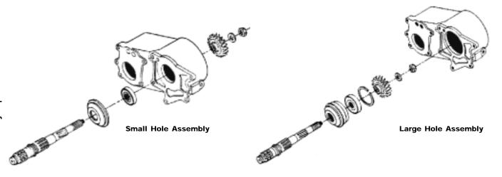
**SPLINES:** All Jeeps and Scouts used a 6 spline input gear except the following applications: Years 1969 to 1971 Jeeps with a T14 transmission used a 10 spline input. Jeeps with an AMC TH400 used a special 15 tooth drive gear. Scout transfer cases used with an automatic were always 23 spline. (*Note:* On Scouts, we recommend you verify your input spline count before ordering parts.)
