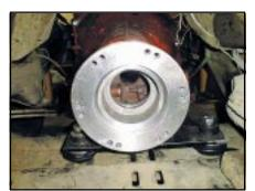
The Atlas will bolt in one of the two rotations on the adapter. We rotated ours almost flat to give us optimum ground clearance.
