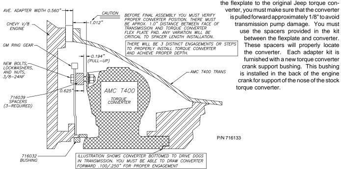
is pulled forward approximately 1/8" to avoid transmission pump damage. You must use the spacers provided in the kit between the flexplate and converter. These spacers will properly locate the converter. Each adapter kit is
