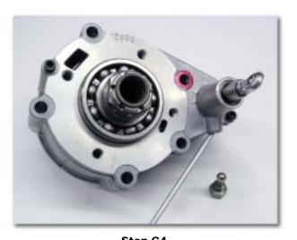
**Step C4**Remove the shift detent screw, ball and spring.
