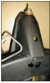
These are the stock frame holes used by Advance Adapters. The lower hole is used to bolt the cradle from the outside of the frame.
