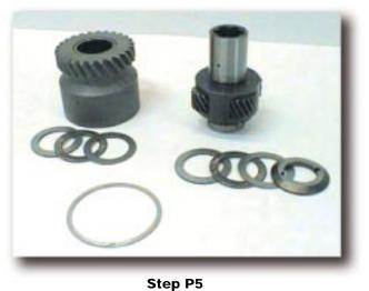
Thoroughly clean & inspect all parts for wear. Replace if necessary.
