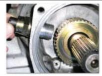
P/N 716073 fits in the main case of a 4L60E transmission and provides a voltage signal.
