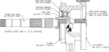
**700R:** This is the first automatic overdrive that GM produced. Introduced in 1982, this transmission was offered in two different bellhousing / case designs (60 & 90 degree bolt
