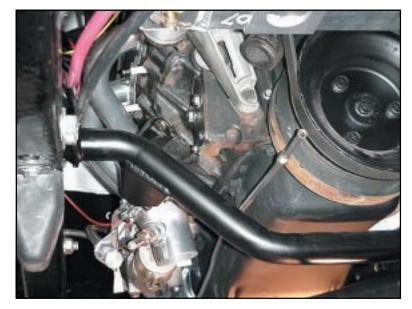
15 We've found that using a deep sump oil pan will cause interference with the crossmember mount; however, a stock oil pan works well.
