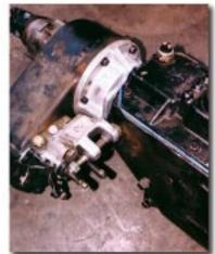
**D. Clutch Linkage:** Both Jeep 4 cylinder engines have been equipped with hydraulic clutch controls. When converting to a Chevy small block and using our full bellhousing, we utilize the Iron Duke slave cylinder. This slave cylinder mounts directly to our conversion bellhousing.
