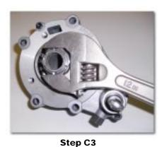
Remove the nut using a 12" adjustable wrench. The shift fork must be at the rear of the case, locking the unit in the overdrive position before the nut can be removed.
