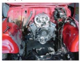
**Universal Motor Mounts:** The universal mounts we manufacture are a high quality mounting system. The "L" brackets in these kits are made out of 3/8" material and designed to handle any style of driving. These universal mounts allow for lateral and vertical placement in the frame rail to maximize you drivetrain fit. The installation of these mounts will require the removal of you stock engine mounts.
