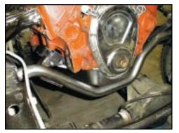
The engine is bolted in using the stock GM mounts provided by Advance Adapters.
