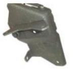
(Brkt. #3) Jeep# 53004278 This bracket is normally used with the AX4 & AX5 transmission.
