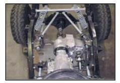
The transmission, adapter, and Atlas are a fairly short combination with an overall length of 38.1". This allows for a 22.5" driveshaft in the rear and a 31" shaft in the front.
