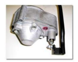
Both above photos illustrate the shift rod installation on the Saturn Overdrive. The shift rod must remain in close proximity to the overdrive unit for proper floorboard clearance. The configuration of some of the shifter rods are to avoid transfer case shifter lever interference.
