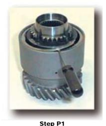
Using a small flathead screwdriver, remove the snap ring from the gear housing.
