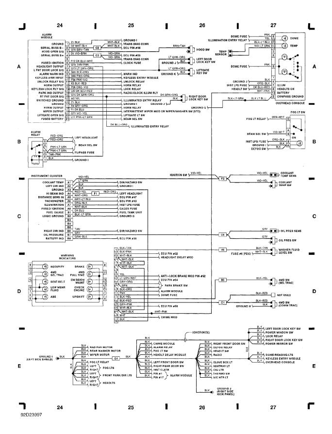
Fig. 8: Accessories & Keyless Entry Module (Grids 28-31) (p. 8) 1992 Jeep Cherokee
