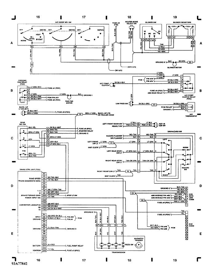
WIRING DIAGRAMS Fig. 6: Wiper/Washer Switches, Stop Light Switch (Grids 20-23) (p. 6) 1993 Jeep Cherokee
