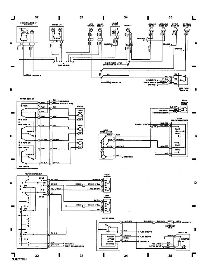
WIRING DIAGRAMS Fig. 10: Power Mirror, Window Switches & Taillights (Grids 36-39) (p. 10) 1993 Jeep Cherokee
