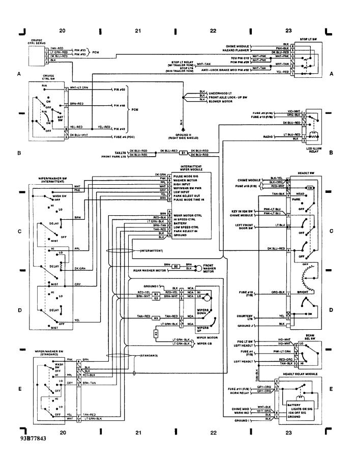
WIRING DIAGRAMS Fig. 7: Instrument Cluster (High Line), (Low Line) (Grids 24-27) (p. 7) 1993 Jeep Cherokee
