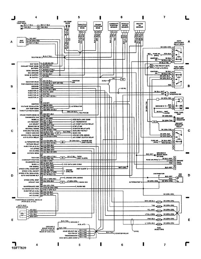
WIRING DIAGRAMS Fig. 3: Ignition Switch (Grids 8-11) (p. 3) 1993 Jeep Cherokee
