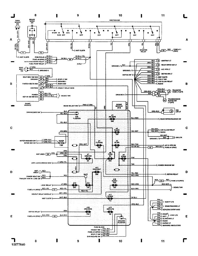
WIRING DIAGRAMS Fig. 4: Anti-Lock Brake Module, ABS Pump Motor (Grids 12-15) (p. 4) 1993 Jeep Cherokee
