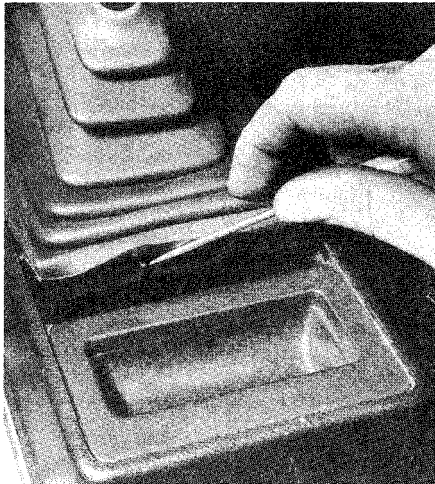
17.3a Pry up on the corner of the transmission shift boot to detach it (manual transmission shown, automatic transmission similar)
