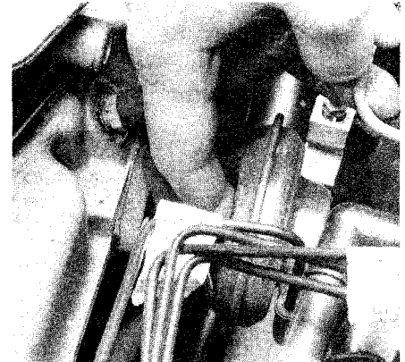
42.2 Move the EGR valve diaphragm in and out to make sure it isn't stuck
