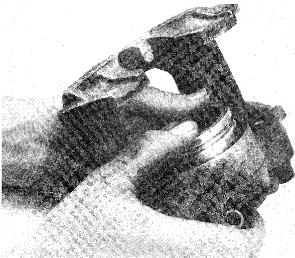
4.15 When installing the piston, make sure it doesn't become cocked in the caliper bore while pushing it down
