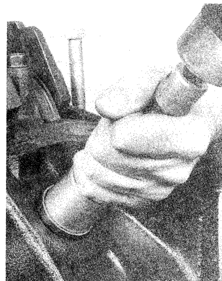
14.10 A large socket on an extension can be used to drive the new soft plugs into the bores
