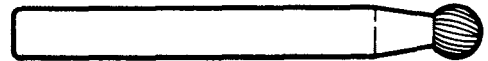
8.17 Use a 3/16-inch diameter cutter to form a groove in the manifold
