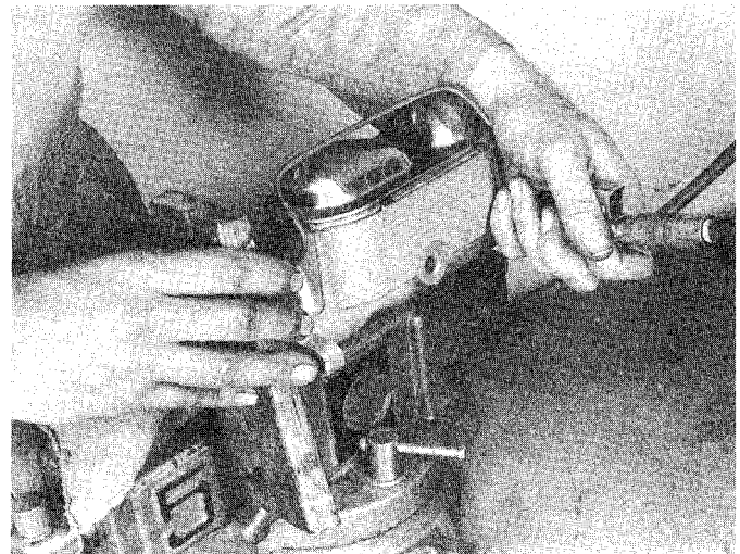
8.9 Eject the secondary piston assembly by applying compressed air to the secondary brake line port. While doing this, cover the opening in the cylinder with a piece of wood to serve as a shield — only apply enough air pressure to ease the piston out!
