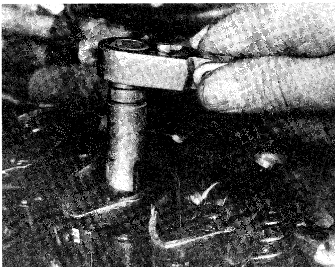
5.2 Go back and forth between the intake and exhaust rocker arms, loosening each bolt 11/4-turn at a time
