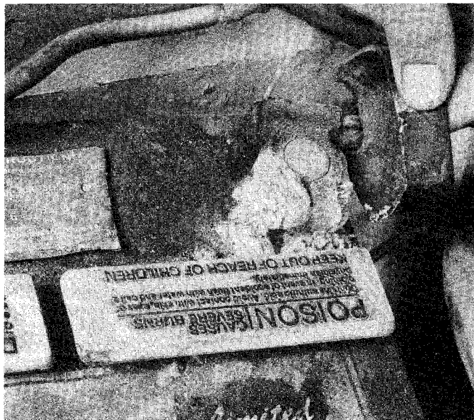
8.8a Battery terminal corrosion usually appears as light, fluffy powder
