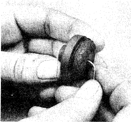
40.11 A paper clip can be used to clean the CCV system orifice
