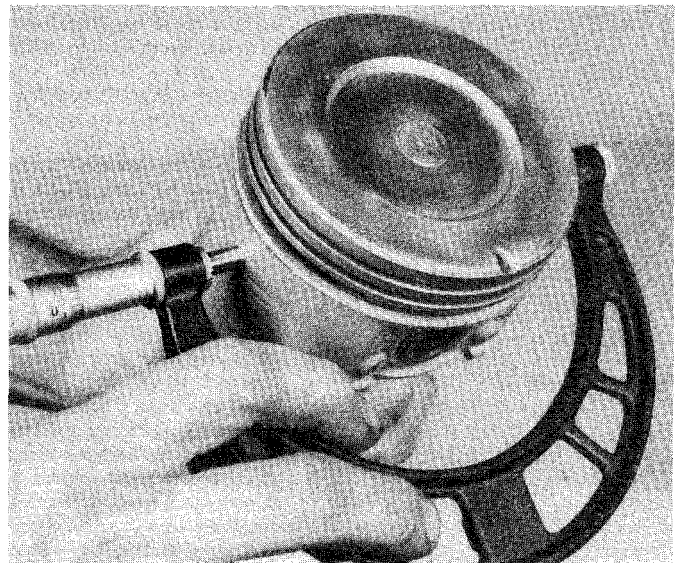
17.11a Measure the piston diameter at a 90° angle to the piston pin and in line with it
