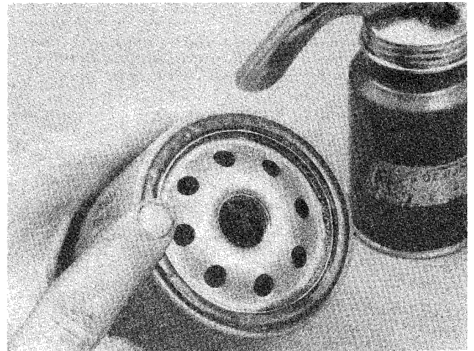
12.18 Lubricate the gasket with clean engine oil before installing the filter on the engine
