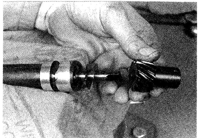
12.11b Remove the driven gear and spacer washers from the end of the shaft, making sure to note the order in which you remove any spacers
