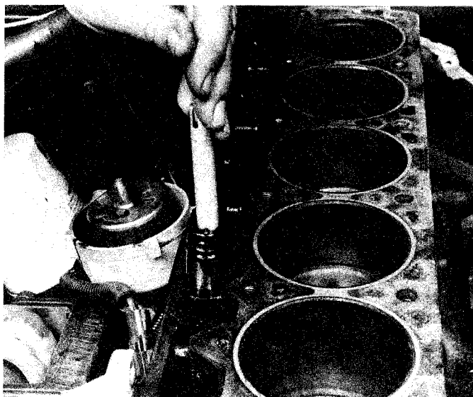
14.9 Remove the lifters with a magnetic pick-up tool (shown here) or a special lifter removal tool
