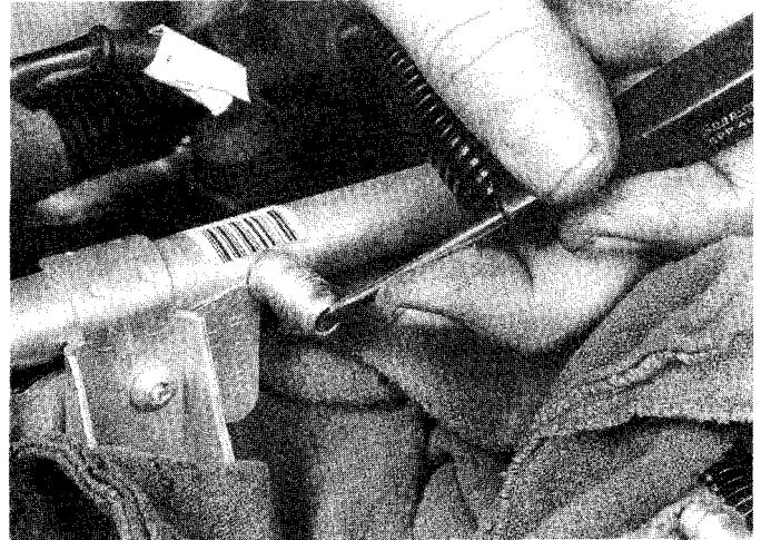
2.7 . . . then depress the valve in the test port with a small screwdriver or pin punch — wear safety goggles during pressure relief to protect your eyes from spraying fuel
