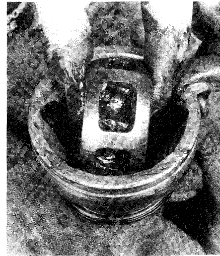
16.13 Tilt the inner race and cage 90-degrees, then align the windows in the cage with the lands and rotate the inner race up and out of the outer race
