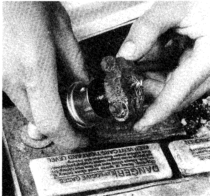
8.8d When cleaning the cable clamps, all corrosion must be removed (the inside of the clamp is tapered to match the taper on the post, so don't remove too much material)
