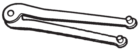
Remover/Installer, Steering Plug C-4381
