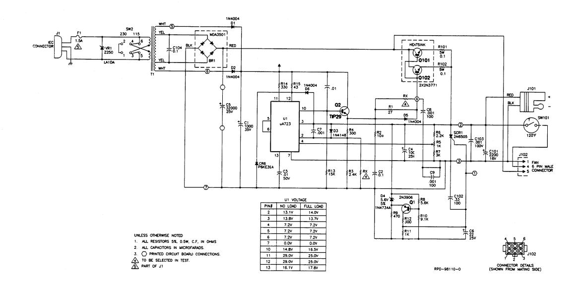
NOTES: 1. THE HPN9041 POWER SUPPLY IS MADE BY ASTRON, AND IS USED IN THE GR400 X-PAND REPEATERS.
