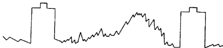
Figure 4—Normal Video and Sync Signal.
