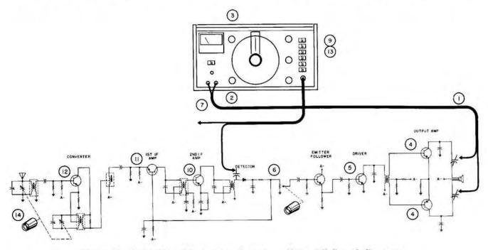
Figure 7. Typical Troubleshooting Technique Using RF Signal Generator
