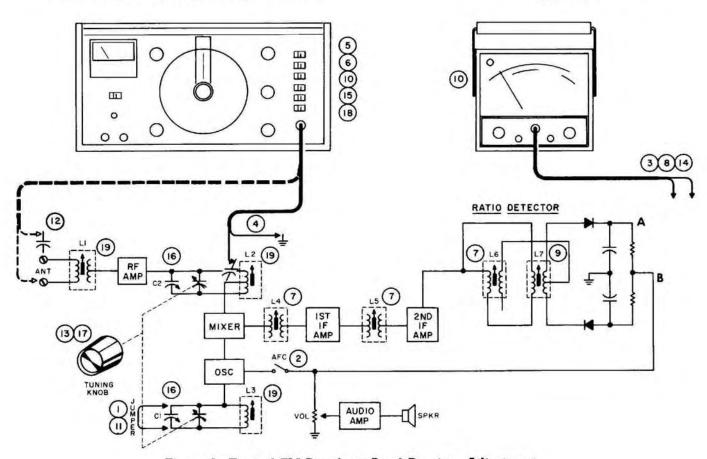
Figure 6. Typical FM Broadcast Band Receiver Adjustment
