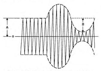
Figure 3. Amplitude Modulation Percentage
