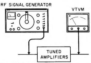
At  $f_c$  the VTVM reads maximum. At  $f_1$  and  $f_2$  the VTVM reads  $\frac{max}{2}$  (—6 dB) Bandwidth =  $f_2$  —  $f_1$
