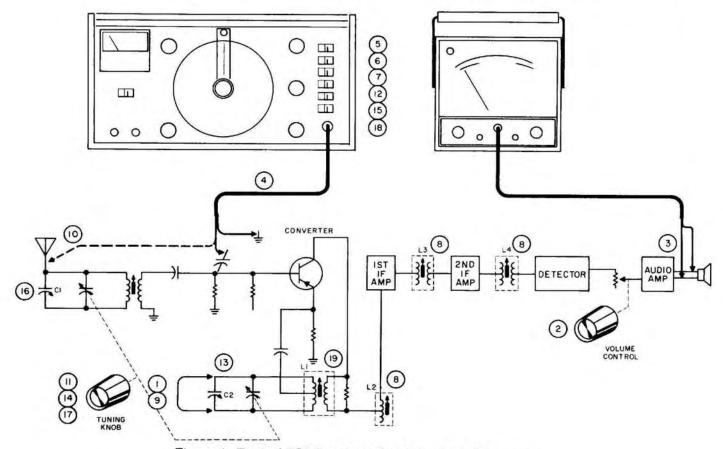
Figure 4. Typical AM Broadcast Band Receiver Alignment
