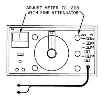
Figure 2. Typical Example, Setting Signal Level
