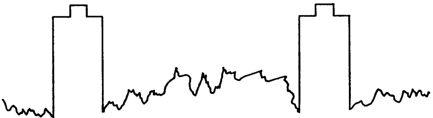
Figure 7. Normal Video and Sync Signal
