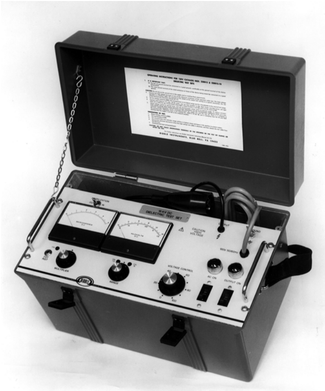
Figure a: The Megger Catalog No. 220015 DC Dielectric Test Set
