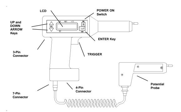
Figure 4-4: Receiver controls, connectors, and indicators
