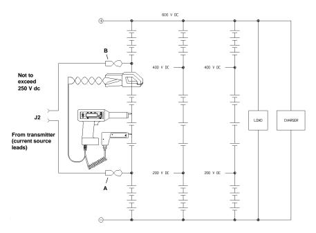
Figure 5-2: Sectioning a battery system greater than 275 V
