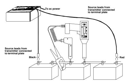
Figure 4-5: BITE 2/2P transmitter connected to the battery
