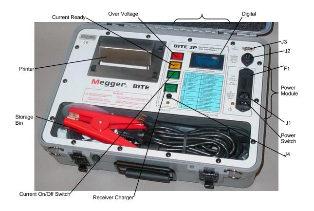
Figure 3-2: BITE 2P transmitter
