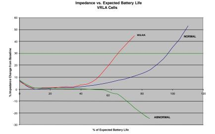
Figure 7-1: Generic curve of impedance vs. cell life
