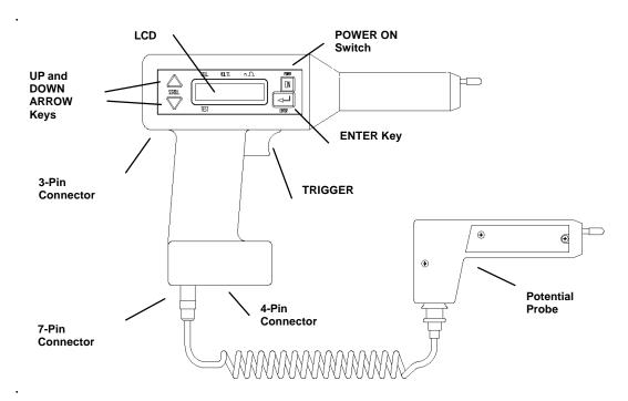
Figure 3-4: Receiver controls, connectors, and indicators
