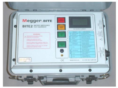
Figure 1-1: BITE 2 instrument
