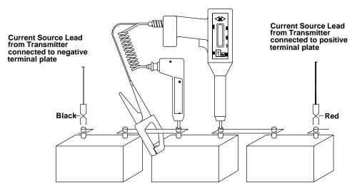
Figure 4-6: Receiver and potential probe positioned on top of battery cell terminals
