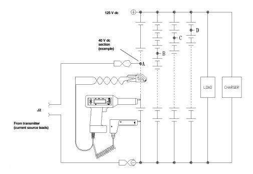
Figure 5-3: Sectioning a parallel string of cells
