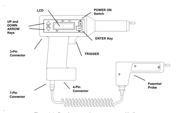
Figure 4-1: Receiver controls, connectors and indicators
