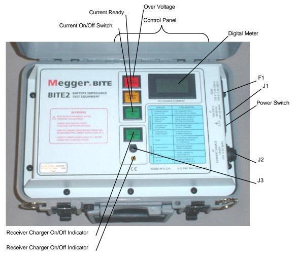
Figure 3-1: BITE 2 transmitter
