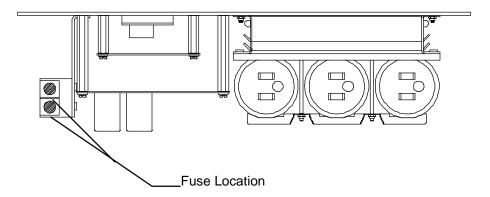
Figure 9-3: BITE 2P transmitter secondary fuses (front view)
