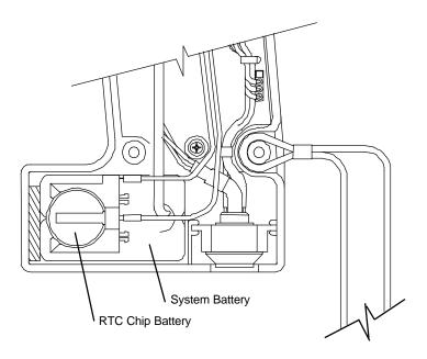
Figure 9-1: RTC battery "piggybacks" the system battery
