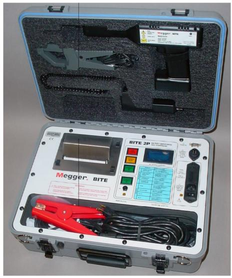
Figure 1-2: BITE 2P instrument
