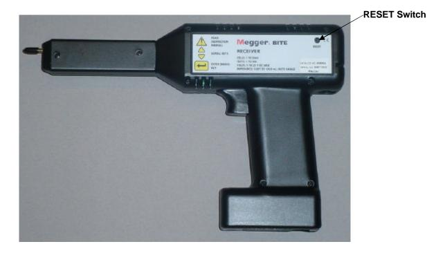
Figure 3-9: Receiver RESET switch
