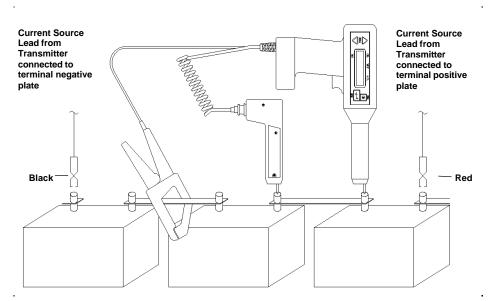
Figure 4-7: Receiver and potential probe positioned on top of battery strap terminals
