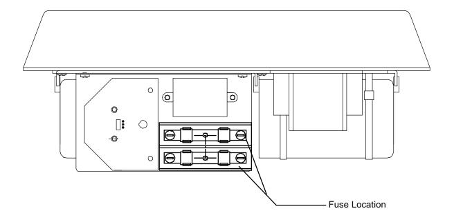
Figure 9-2: BITE 2 transmitter secondary fuses (front view)
