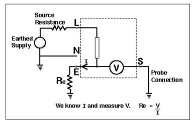
The measurement depends on the position of the probe. The probe must be positioned away from any part of the installation under test, so that it provides a valid reference earth. For a single earth electrode, the distance of 20 m is found to be sufficient. Be careful of secondary earth paths, such as service pipes. The best way to confirm the measurement is to try two probe positions.
