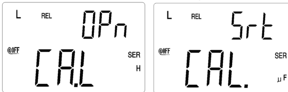
Figure-7. Open/ Short Calibration
