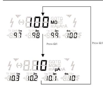
**Figure 4 - The result of a step voltage (SV) test** Test condition: timer defaults to 5 minutes and test voltage defaults to 1000 V.
