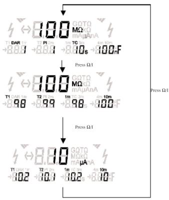
Figure 1 - The result of an insulation resistance test (IR)
