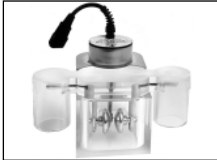
Figure 13. Oil test vessel for ASTM D1816 specification.
