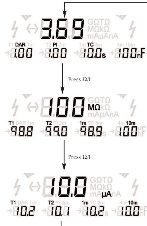
Figure 3 - The result of a dielectric discharge test (DD)
