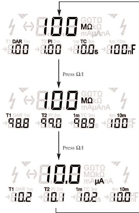
Figure 2 - The result of a polarity index test (PI)
