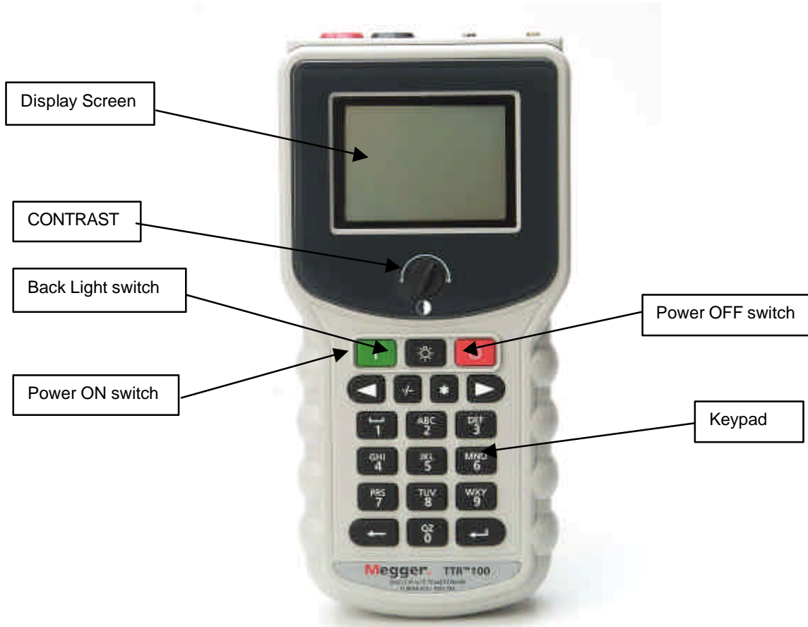
Figure 4-2 Single-Phase TTR Display & Control Panel
