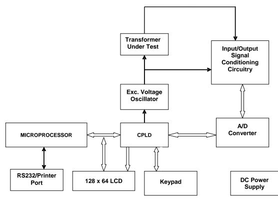
Figure 1-1.TTR25 Test Set Block Diagram
