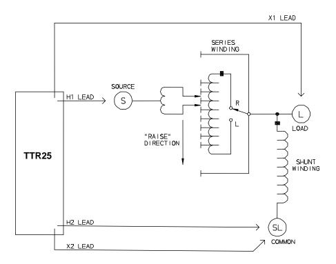
Figure 4-4 Setup for Testing Single-Phase, Type B (Inverted Design) Step Voltage Regulator
