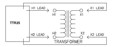
Figure 4-1 Setup for Testing Single-Phase Transformer
