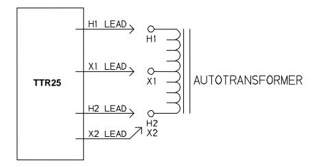
Figure 4-2 Setup for Testing Single-Phase Autotransformer
