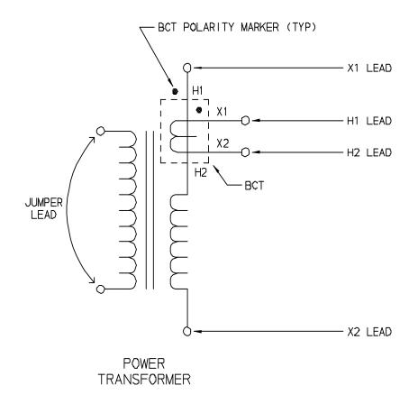
Figure 4-10 Setup for Testing BCT Mounted on Single-Phase Two-Winding Transformer
