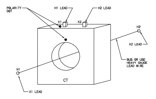
Figure 4-8 Setup for Testing Unmounted Current Transformer
