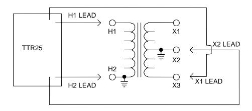
Figure 4-6 Setup for Testing X3 – X2 Winding of Distribution Transformer (H2 and X2 Grounded)
